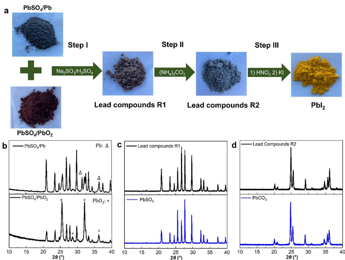
Fig. 1 (a) Lead recycling process from lead-acid battery to  $\text{PbI}_2$ ; (b) XRD patterns of lead-containing compounds from the negative and positive electrodes; (c) XRD patterns of pure  $\text{PbSO}_4$  and lead-containing compounds after the first step; (d) XRD patterns of pure  $\text{PbCO}_3$  and lead-containing compounds after the second step.
