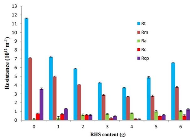
Fig. 9 Resistance,  $R_t$ : total;  $R_m$ : membrane;  $R_a$ : due to absorption;  $R_c$ : due to cake layer;  $R_{cp}$ : due to cake polarization.<sup>54</sup>
