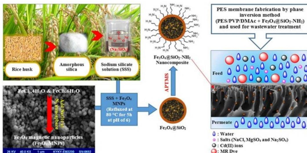
Fig. 5 Graphical representation of the fabrication of  $\text{Fe}_3\text{O}_4@\text{SiO}_2\text{-NH}_2$ -embedded PES membrane and its waste water treatment application.<sup>40</sup>
