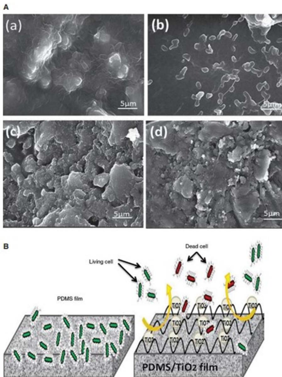
Fig. 7 (A) SEM images of the composite film at different concentrations of  $\text{TiO}_2$ : (a) 0 wt%, (b) 7 wt%, (c) 10 wt%, and (d) 13 wt%. (B) Schematic of antibacterial mechanism of the composite film.<sup>47</sup>
