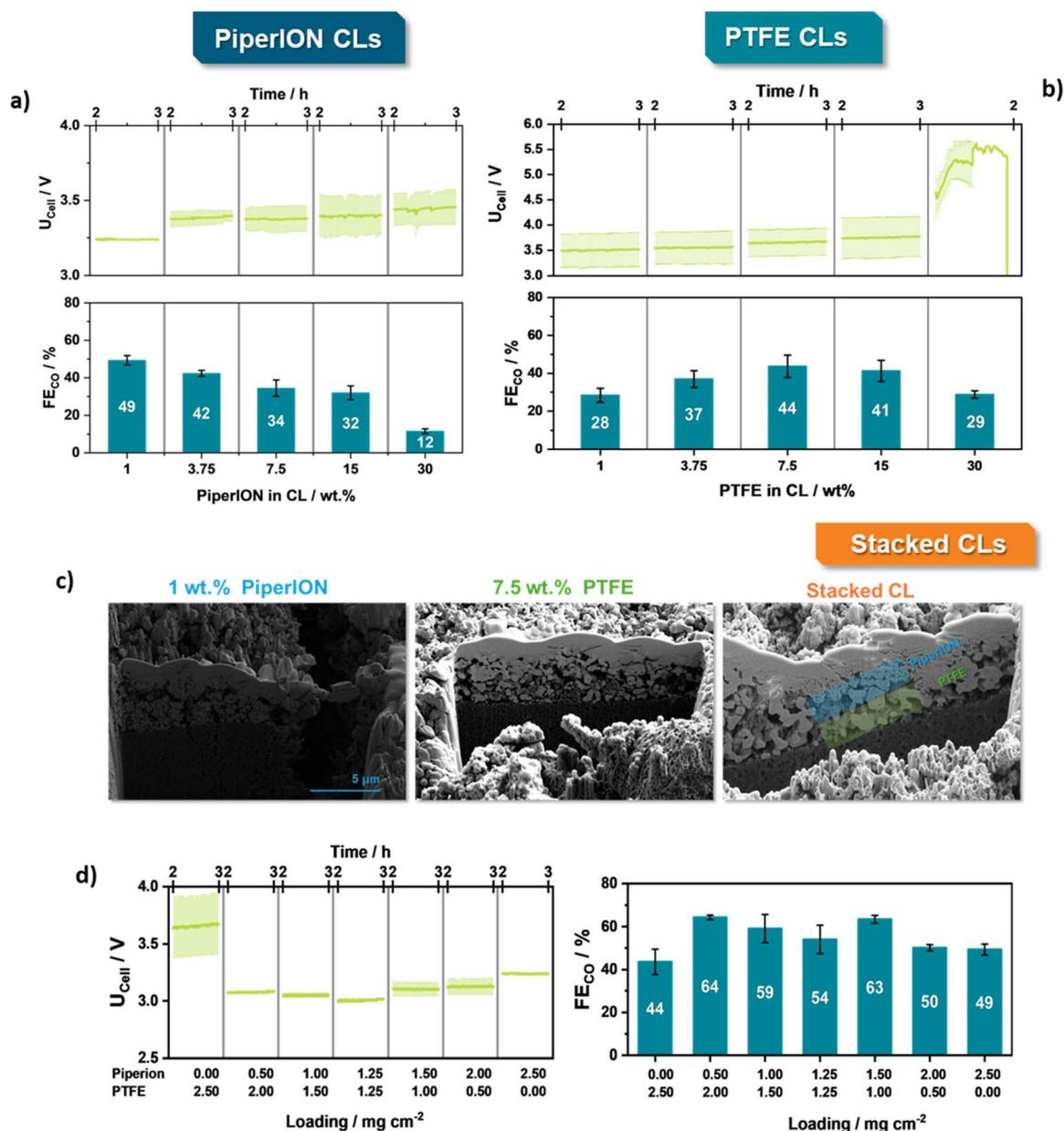
Fig. 3 Electrochemical characterization of the herein presented catalytic layers/GDEs at  $300 \text{ mA cm}^{-2}$  at  $60^\circ \text{C}$  between 2nd and 3rd hour of electrolysis for the PiperION-bound CLs (a), PTFE-bound (b) and stacked (d) CLs. FIB-SEM analysis of the different catalytic layers (c).
