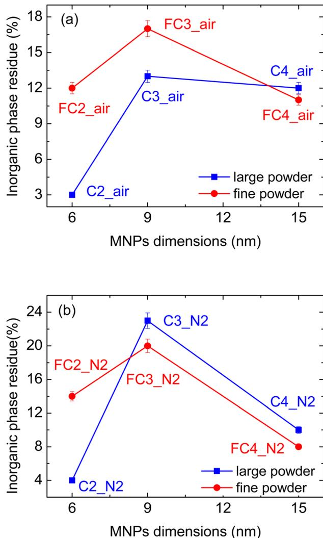
Fig. 5 Inorganic phase residues as a function of the MNPs' dimensions for composites prepared (a) in air and (b) in N<sub>2</sub>.
