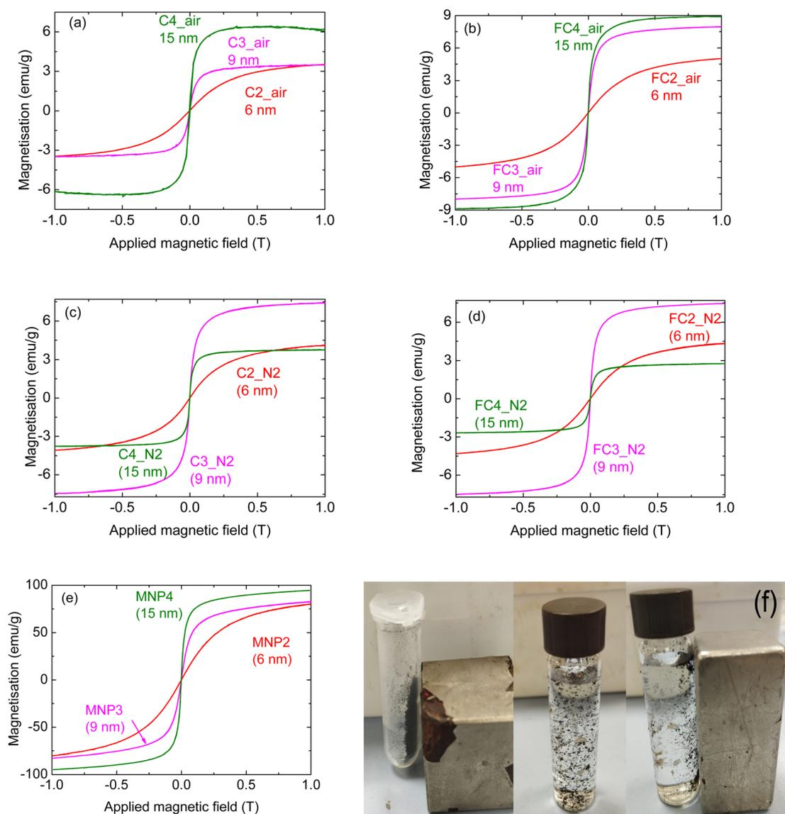
Fig. 4 Magnetisation of the composites prepared with Fe<sub>3</sub>O<sub>4</sub> MNPs of different dimensions, using pyrolysed large cork powder C (a) in air and (c) in N<sub>2</sub>; pyrolysed fine cork powder FC (b) in air and (d) in N<sub>2</sub>; (e) MNPs alone. (f) Photographs of FC4<sub>air</sub> particles in air and in a suspension of water, without and with the presence of an exterior magnet, demonstrating that this material can be magnetically separated.
