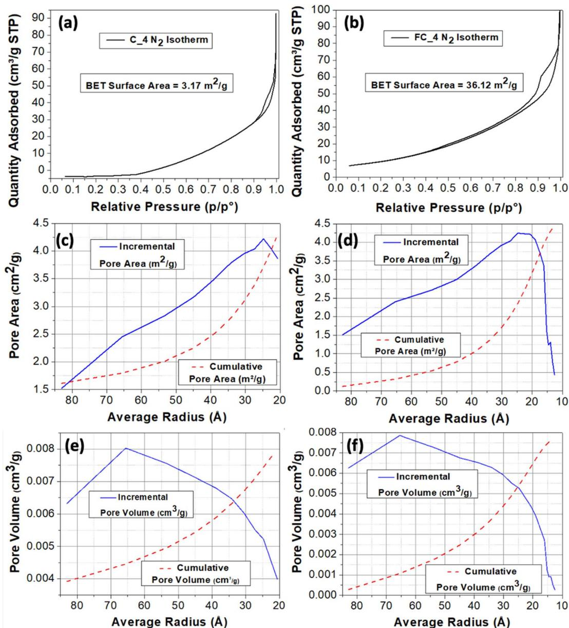
Fig. 6 Specific surface area (SSA) measurements of C<sub>4</sub> (a, c and e) and FC<sub>4</sub> (b, d and f). BET N<sub>2</sub> adsorption/desorption isotherms (a and b), and BJH average pore radius distribution for pore area (c and d) and pore volume (e and f) below 100 Å.
