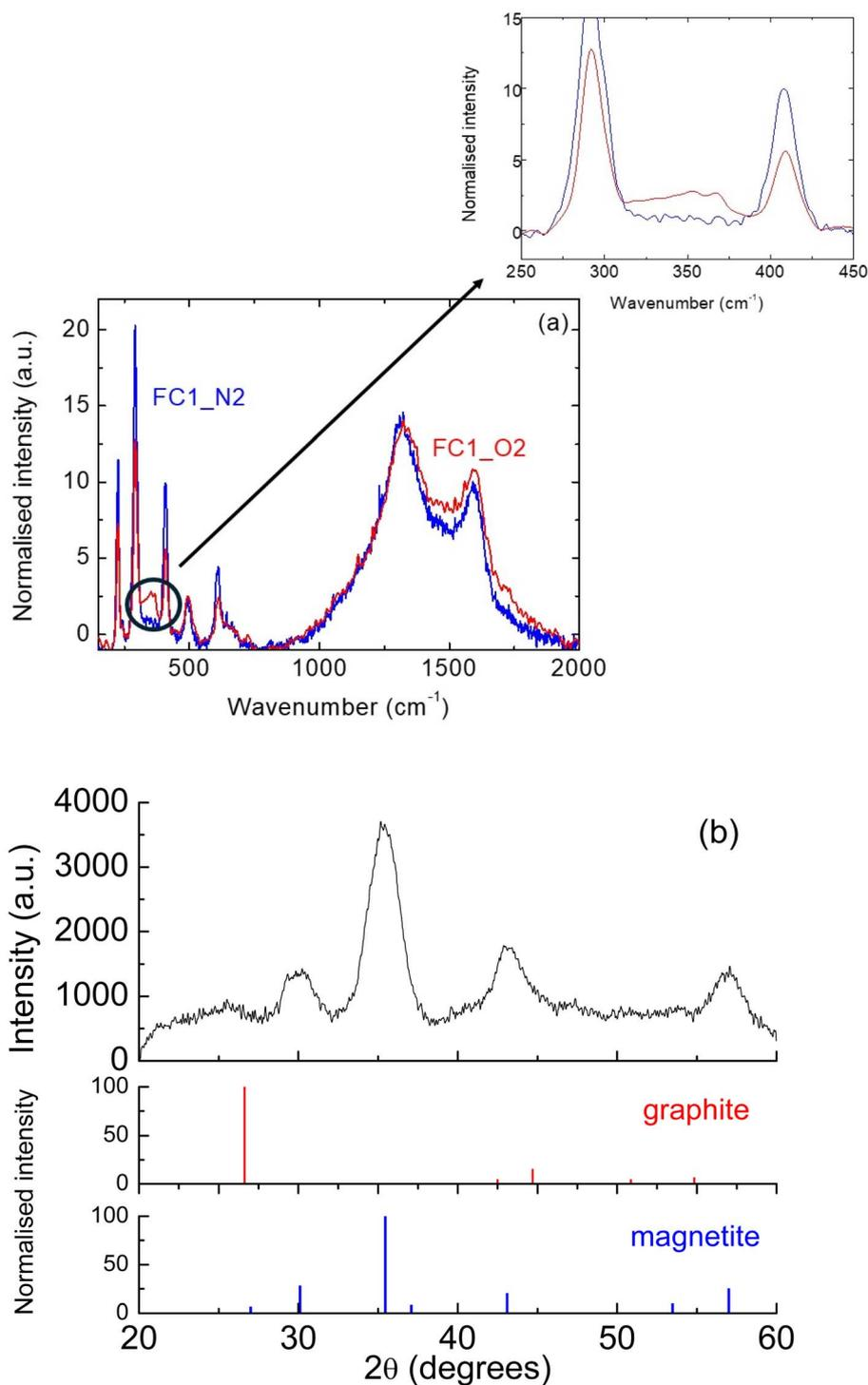
Fig. 2 (a) Raman spectra for samples FC1\_N<sub>2</sub> and FC1\_air; (b) XRD pattern for the sample FC2\_air. The standard XRD patterns used for identification were 75-2078 for  $\alpha$ -graphite and 19-629 for magnetite.
