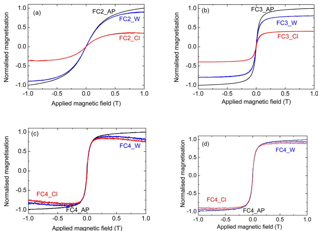
Fig. 8 Stability of the composites prepared using pyrolysed fine cork powder and (a) **MNP2**, (b) **MNP3**, and (c) **MNP4**, (d) **MNP4** after diamagnetic component subtraction. The curves indicated with AP, W and CI correspond to the material as prepared, and left in water and in chloroform, respectively, for 24 hours.
