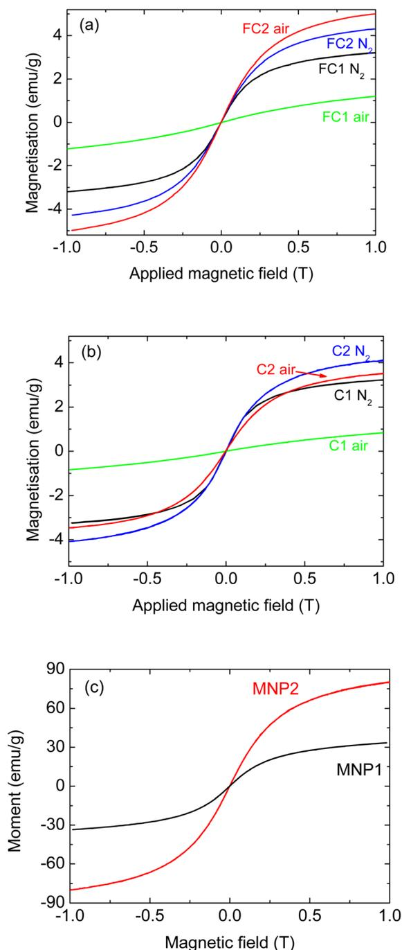
Fig. 1 Magnetisation for composites prepared with MNP1 (6 nm  $\text{ZnFe}_2\text{O}_4$ ) and MNP2 (6 nm  $\text{Fe}_3\text{O}_4$ ), (a) with fine pyrolysed cork powder FC, (b) large pyrolysed cork powder C, and (c) MNPs alone.
