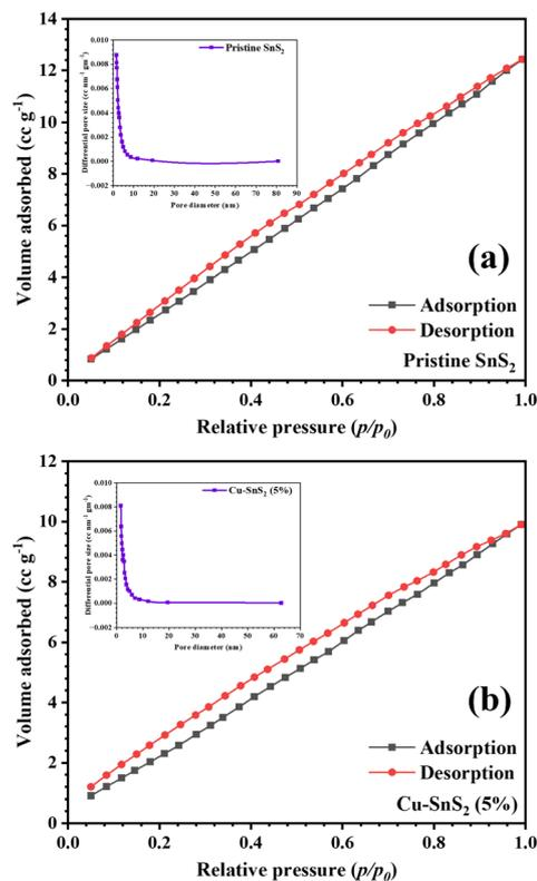
Fig. 3 N<sub>2</sub> adsorption–desorption isotherms for (a) pristine and (b) 5% Cu-doped SnS<sub>2</sub> with their respective pore size distributions given in the insets.
