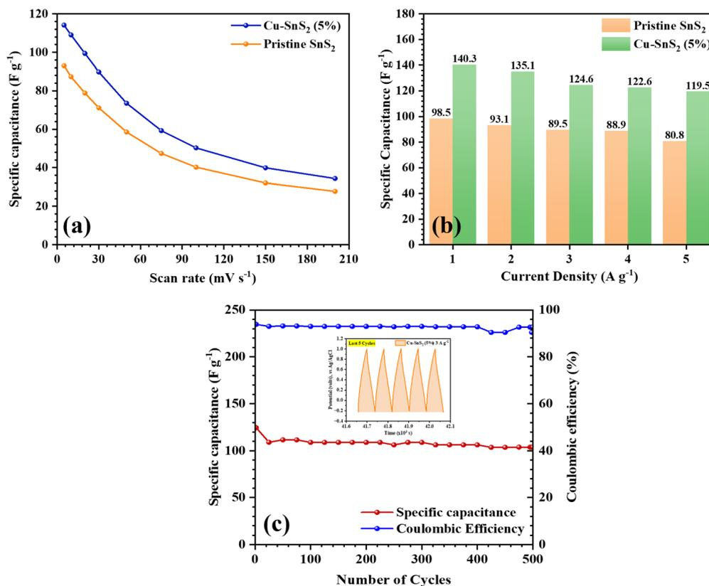
Fig. 7 Variation of specific capacitance with (a) scan rates and (b) current densities. (c) Cycling stability of the 5% Cu-doped SnS<sub>2</sub> electrode at 3 A g<sup>-1</sup> with the last 5 charge-discharge cycles given in the inset.
