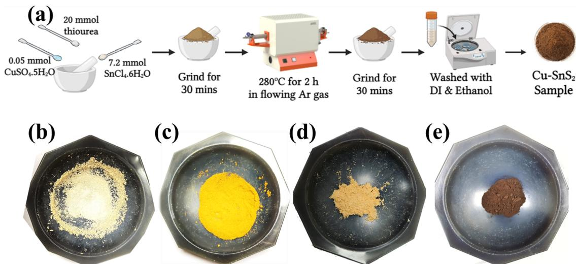
Fig. 1 (a) Schematic illustration of the procedure for synthesizing Cu-doped SnS<sub>2</sub> nanoflakes. (b–e) Comparative images illustrating the visible changes in SnS<sub>2</sub> and Cu-SnS<sub>2</sub> nanoflakes before and after heating in an inert furnace. (b) SnS<sub>2</sub> before heating, (c) SnS<sub>2</sub> after heating, (d) Cu-SnS<sub>2</sub> before heating, and (e) Cu-SnS<sub>2</sub> after heating.
