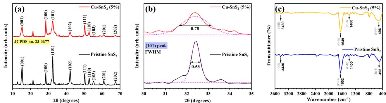
Fig. 2 (a) XRD profiles of pristine and 5% Cu-doped SnS<sub>2</sub> with (b) magnified view of (101) peak broadening. (c) FTIR spectra of pristine and 5% Cu-doped SnS<sub>2</sub>.
