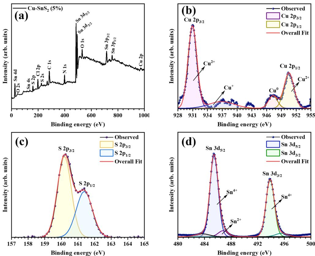
Fig. 5 (a) XPS survey spectrum for 5% Cu-doped SnS<sub>2</sub> and XPS spectra showing peaks for (b) Cu 2p, (c) S 2p and (d) Sn 3d.
