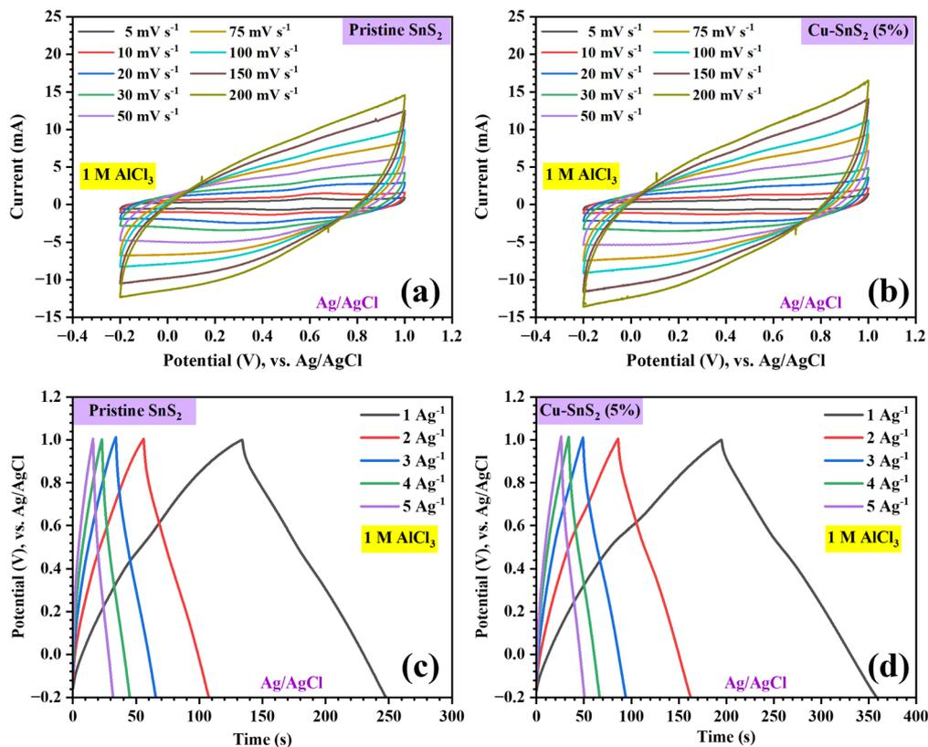
Fig. 6 Cyclic voltammograms for (a) pristine and (b) 5% Cu-doped SnS<sub>2</sub> and charge-discharge curves of (c) pristine and (d) 5% Cu-doped SnS<sub>2</sub>.
