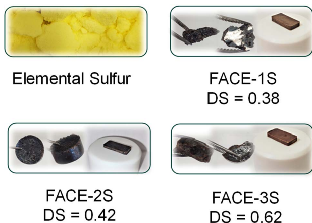
Fig. 1 Optical appearance of the synthesized high sulfur content composite materials FACE-1S, FACE-2S, and FACE-3S.
