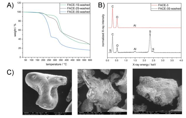
Fig. 2 (A) TGA curves of FACE-1S-washed (green line), FACE-2S-washed (black line), and FACE-3S-washed (blue line) from 25 to 600 °C with a heating rate of 10 K min<sup>-1</sup> under a nitrogen flow. (B) EDX spectra of FACE-3 (red line) and FACE-3S-washed (black line). (C) SEM pictures of FACE-1S-washed (middle), FACE-2S-washed (right) and FACE-3S-washed (left).
