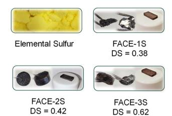
Fig. 1 Optical appearance of the synthesized high sulfur content composite materials FACE-1S, FACE-2S, and FACE-3S.
