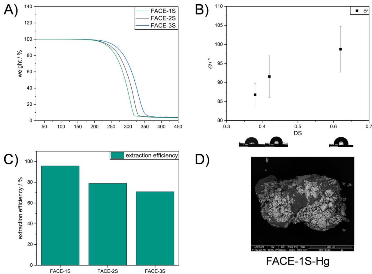
**Fig. 3** (A) TGA curves of FACE-1S (green line), FACE-2S (black line), and FACE-3S (blue line). (B) Static WCA measurements of FACE-1S, FACE-2S, and FACE-3S. (C) Mercury removal efficiency of FACE-1S, FACE-2S, and FACE-3S from an aqueous  $\text{HgCl}_2$  solution ( $1.00 \text{ mg L}^{-1}$ ) after 24 h at ambient temperature. (D) Backscattered electron image of FACE-1S after mercury uptake *via* SEM.
