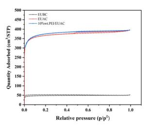
Fig. 6 N<sub>2</sub> adsorption-desorption isotherms of the EU series.
