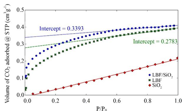
Fig. 4 Isotherms for CO<sub>2</sub> adsorption at room temperature.
