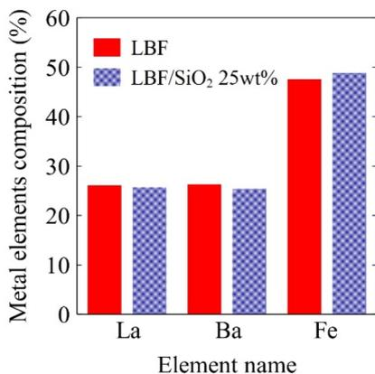
Fig. 1 Metal elemental compositions of fresh samples in bulk calculated from XRF results, red solid bar is LBF result, and blue dotted bar is for LBF/SiO<sub>2</sub> 25 wt%.
