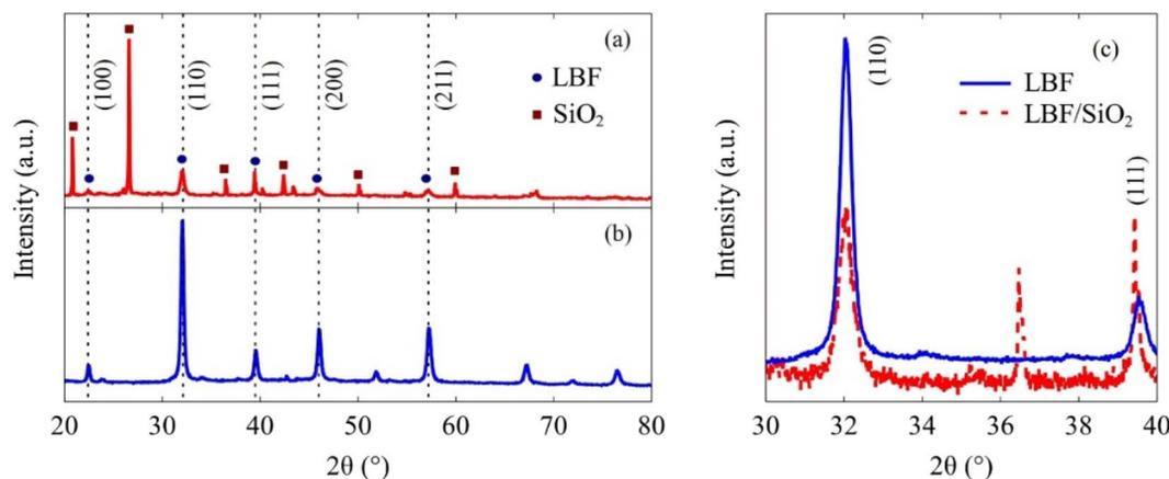
Fig. 2 XRD results of synthesized samples. (a) LBF/SiO<sub>2</sub>, circular marker denotes the crystal planes from LBF, and rectangular marker denotes the crystal planes from SiO<sub>2</sub>. (b) LBF. (c) Detailed results in the  $2\theta$  range of 30 to 40°.
