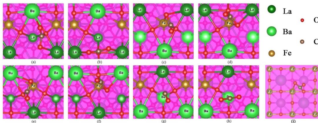
Fig. 7 The CO<sub>2</sub> adsorption on each configuration. (a) & (b) are the adsorption results of LBF-111(LaBa–La). (c) & (d) are the adsorption results of LBF-111(LaBa–Fe), (e) & (f) are the adsorption results of LBF-111(BaLa–Fe). (g) & (h) are the adsorption results of LBF-111(BaLa–Ba), C–O<sub>b</sub> in (g) is not marked because it is away to the ideal range. (i) is the adsorption result of LBF-100(Fe–O).
