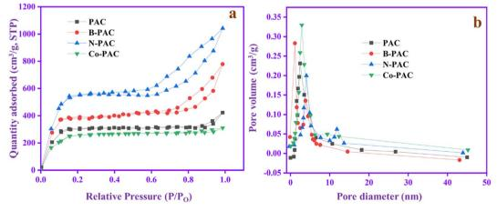
Fig. 5 (a). N<sub>2</sub> adsorption-desorption isotherms and (b) pore size distribution of PAC, B-PAC, N-PAC, and Co-PAC.
