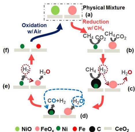
Fig. 14 Proposed reaction mechanism for Fe–Ni physical mixture. Reprinted with permission.<sup>62</sup> Copyright 2016 John Wiley and Sons.
