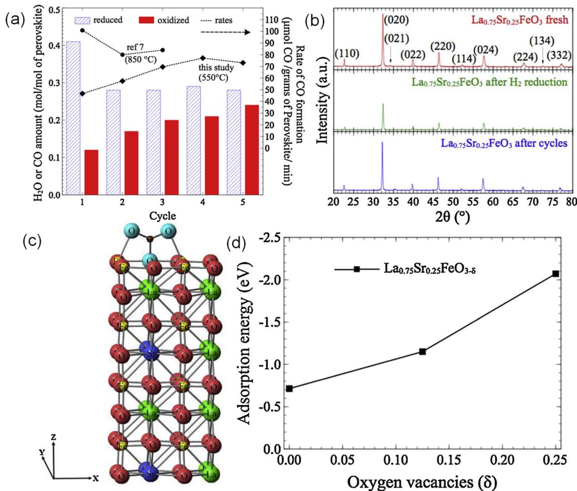
Fig. 2 (a) RWGS-CL performance of  $\text{La}_{0.75}\text{Sr}_{0.25}\text{FeO}_3$  (LSF) at 823 K. (b) XRD data of the LSF powder during RWGS-CL. (c) Adsorption energies of  $\text{CO}_2$  on (1 0 0) facet of stoichiometric LSF. (d) Change of  $\text{CO}_2$  adsorption energy with oxygen vacancies ( $\delta = 0, 0.125, 0.250$ ). Reprinted with permission.<sup>38</sup> Copyright 2014 Elsevier.
