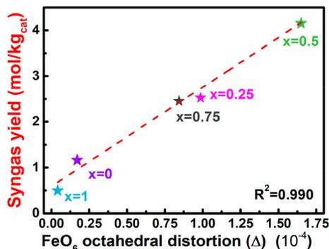
Fig. 8 Linear relation between the syngas yield and the FeO<sub>6</sub> octahedral distortion in La<sub>1-x</sub>Ce<sub>x</sub>FeO<sub>3</sub>. Reprinted with permission.<sup>64</sup> Copyright 2020 American Chemical Society.
