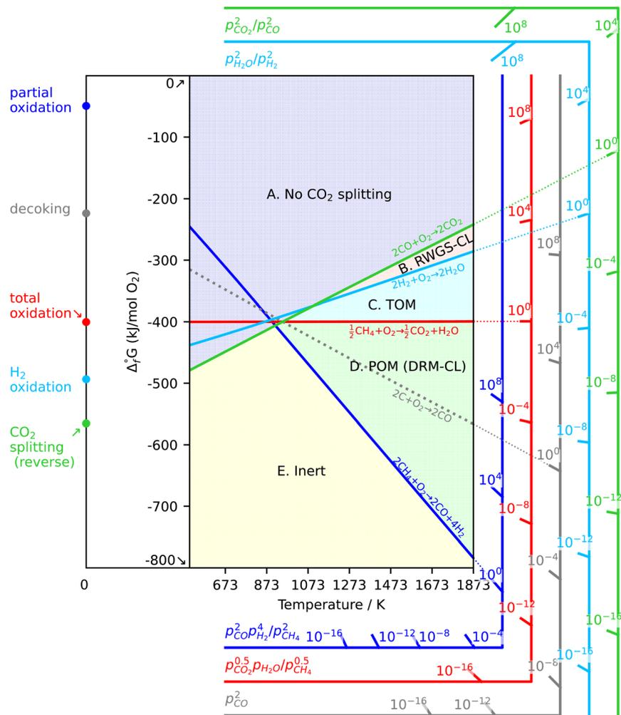
Fig. 17 Different zones for chemical looping processes. Reaction line 1:  $2\text{CO} + \text{O}_2 = 2\text{CO}_2$ . Reaction line 2:  $2\text{H}_2 + \text{O}_2 = 2\text{H}_2\text{O}$ . Reaction line 3:  $\frac{1}{2}\text{CH}_4 + \text{O}_2 = \frac{1}{2}\text{CO}_2 + \text{H}_2\text{O}$ . Reaction line 4:  $2\text{CH}_4 + \text{O}_2 = 2\text{CO} + 4\text{H}_2$ .
