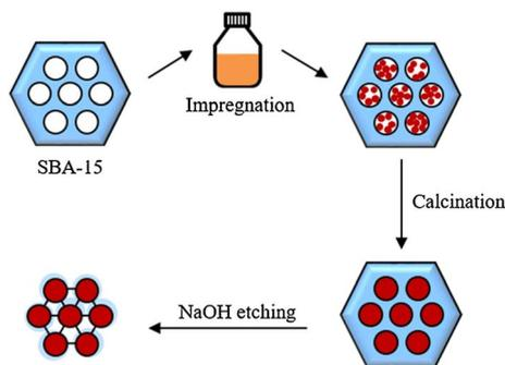
Fig. 3 Synthesis method of nanocast mesoporous LSF. Reprinted with permission.<sup>44</sup> Copyright 2021 Elsevier.
