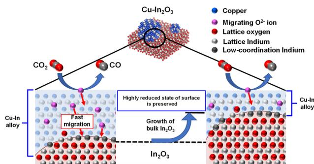
Fig. 6 Proposed mechanism of  $CO_2$  splitting on the reduced  $Cu-In_2O_3$ . Reprinted with permission.<sup>58</sup> Copyright 2021 RSC Publishing.
