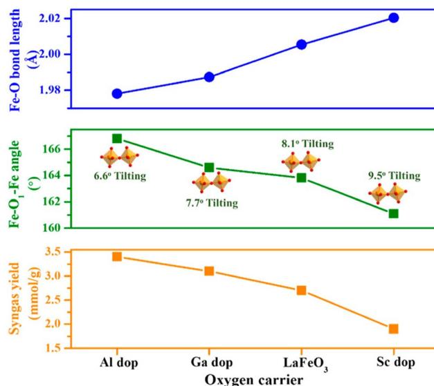
Fig. 9 Correlation between structural distortion and the CH<sub>4</sub> conversion performance in the first cycle over LaFe<sub>0.8</sub>M<sub>0.2</sub>O<sub>3</sub>. Reprinted with permission.<sup>67</sup> Copyright 2022 American Chemical Society.
