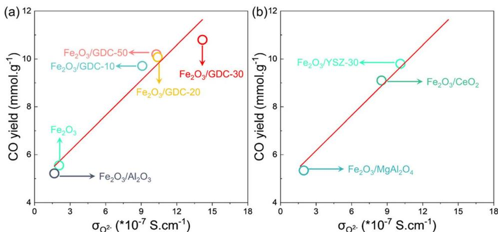
Fig. 5 (a) Fitted linear curve relation between  $O^{2-}$  conductivity and CO yield to predict activity of supported  $Fe_2O_3$  and (b)  $O^{2-}$  conductivity and CO yield for reference samples to validate the fitted curves. Reprinted with permission.<sup>57</sup> Copyright 2020 American Chemical Society.
