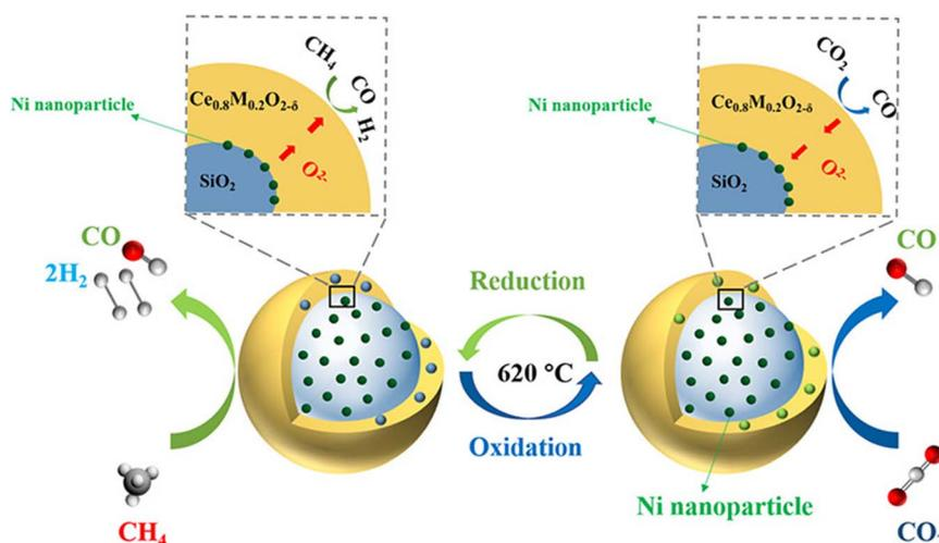
Fig. 12 Proposed reaction model for sandwich and core-shell Ni-phyllsilicate@Ce<sub>0.8</sub>M<sub>0.2</sub>O<sub>2-δ</sub> (M = Fe, Co, Ni) composites. Reprinted with permission.<sup>87</sup> Copyright 2022 Elsevier.
