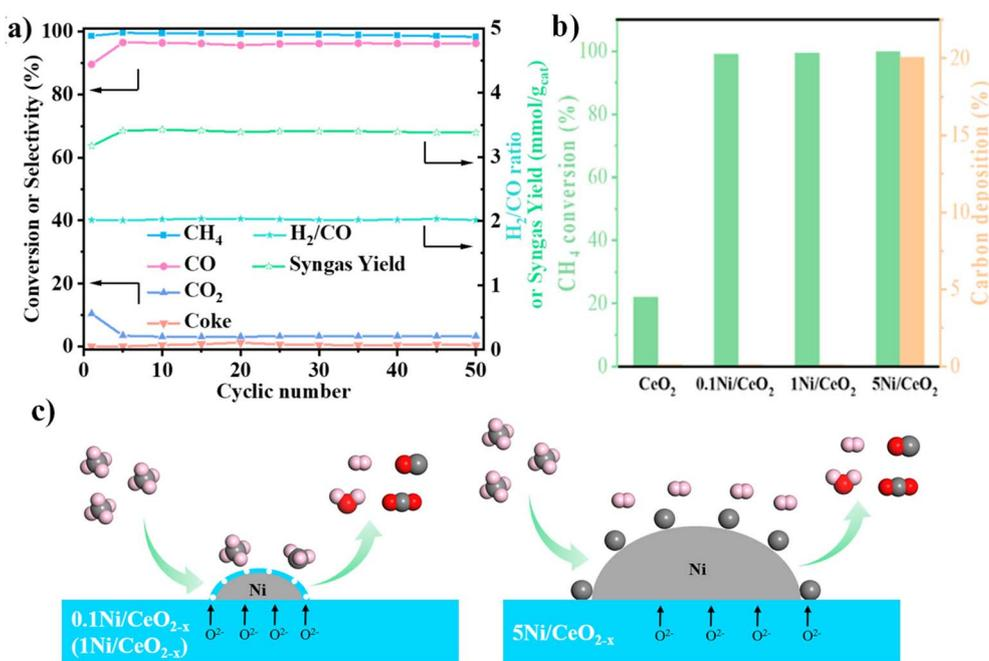
Fig. 11 (a) Performance over 0.1Ni/CeO<sub>2</sub> in the partial oxidation of methane step during 50 cycles. (b) Comparison of CH<sub>4</sub> conversion and carbon deposition between CeO<sub>2</sub>, 0.1Ni/CeO<sub>2</sub>, 1Ni/CeO<sub>2</sub> and 5Ni/CeO<sub>2</sub>. (c) Proposed reaction pathways for the reduction step by CH<sub>4</sub> over 0.1Ni/CeO<sub>2</sub> (1Ni/CeO<sub>2</sub>) and 5Ni/CeO<sub>2</sub>. Reprinted with permission.<sup>84</sup> Copyright 2021 American Chemical Society.
