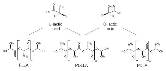
Fig. 2 Molecular structures of PLA's monomeric units, L-lactic acid and D-lactic acid, and their arrangements as PLA's three different stereoisomeric forms: PLLA, PDLLA, and PDLA,
