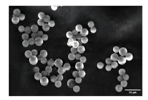
Fig. 22 SEM image of functionalized magnetic dextran microbeads. (The original image has been cropped. Reproduced from ref. 179 under CC-BY.)179
