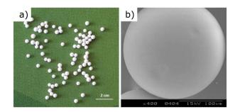
Fig. 3 Example images of PLGA microbeads for a biomedical application: (a) digital photograph and (b) SEM image. (The original image has been cropped. Reproduced from ref. 47 under CC-BY.)<sup>47</sup>
