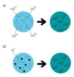
Fig. 16 Simplified representation of (a) external *versus* (b) internal ionotropic gelation using Ca<sup>2+</sup> ions as an example.
