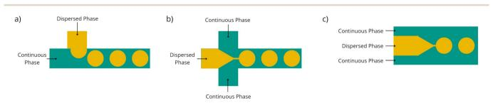
Fig. 13 Representation of different designs for fluidic devices: (a) T-junction device, (b) flow-focusing device, and (c) co-flow device.
