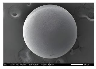
Fig. 1 Scanning electron microscopy image of a polyethylene microbead extracted from a cream-based personal hygiene product. (The original image has been cropped. Reproduced from ref. 33 under CC-BY.)33
