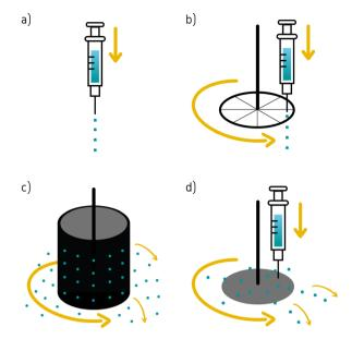
Illustration of various techniques used in the production of cellulose microbeads: (a) dropping, (b) jet cutting, (c) spinning drop atomization, and (d) spinning disc atomization.
