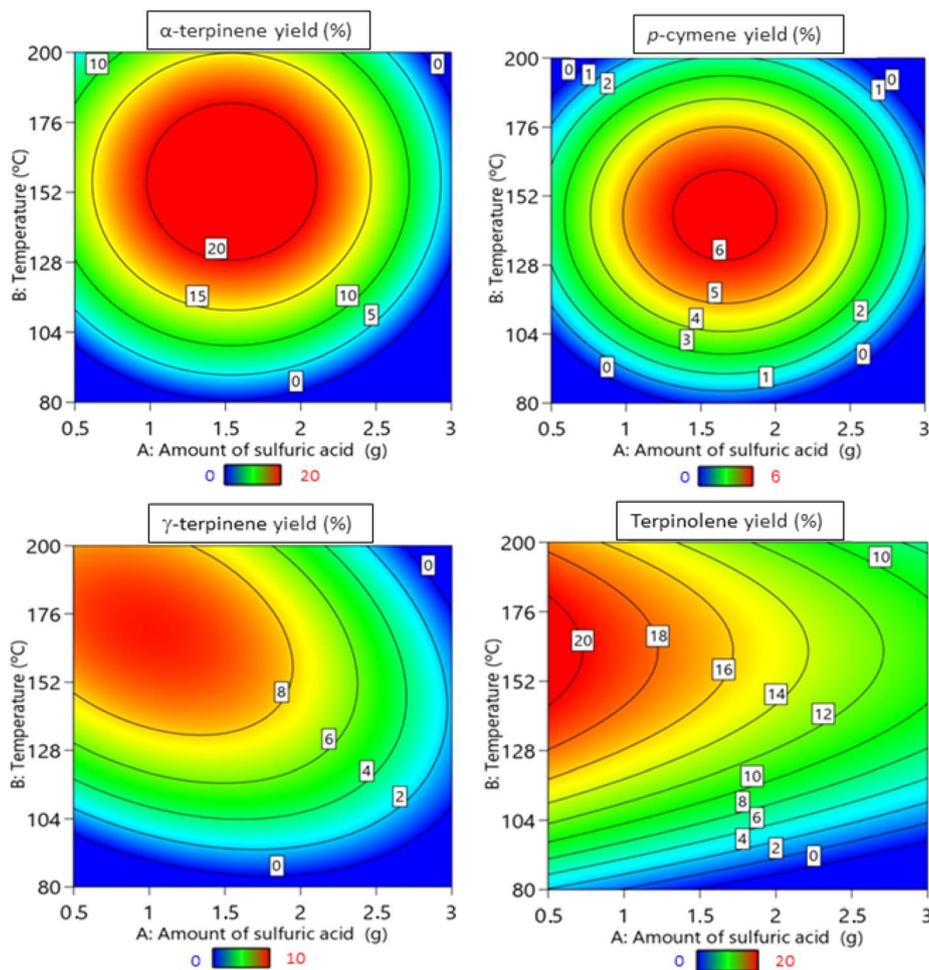
Fig. 4 Response surface obtained in the optimization process of sulfonated carbons through *in situ* carbonization and sulfonation. Effect of temperature and H<sub>2</sub>SO<sub>4</sub> quantity during catalyst preparation on products of limonene isomerization.
