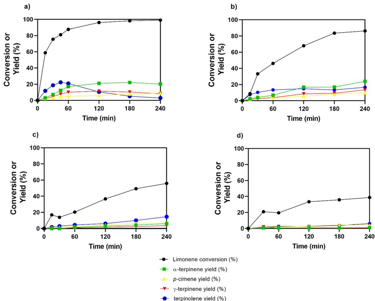
Fig. 6 Recycling test outcomes of limonene isomerization on the optimized sulfonated carbons (catalyst sample produced using 1.4 g of  $\text{H}_2\text{SO}_4$  and a temperature of 155 °C. The experimental setup involved the utilization of 30 mmol of limonene, a catalyst loading of 15% by weight, and a reaction temperature of 150 °C. (a) First cycle, (b) second cycle, (c) third cycle, (d) fourth cycle.
