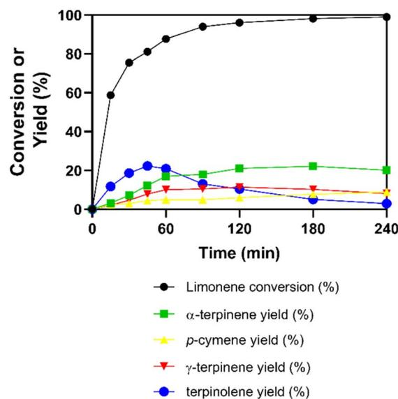
Fig. 5 Catalytic outcomes of limonene isomerization using the optimized sulfonated carbon catalyst (catalyst sample produced using 1.4 g of  $\text{H}_2\text{SO}_4$  and a temperature of 155  $^{\circ}\text{C}$ ). The experimental setup involved the utilization of 30 mmol of limonene, a catalyst loading of 15% by weight, and a reaction temperature of 150  $^{\circ}\text{C}$ .
