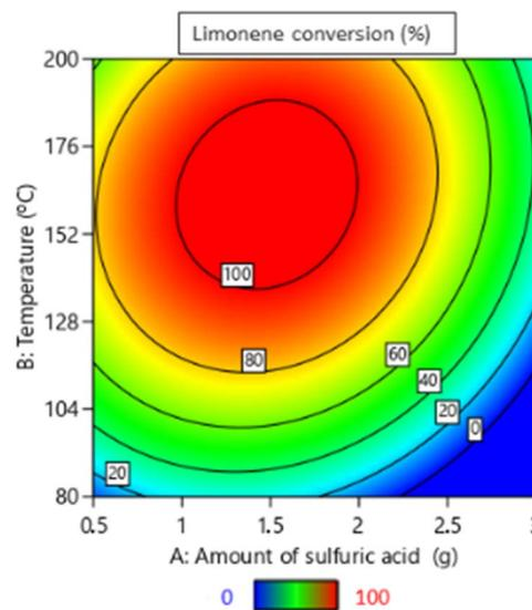
Fig. 3 Response surface obtained in the optimization process of sulfonated carbon catalysts through *in situ* carbonization and sulfonation. Effect of temperature and  $\text{H}_2\text{SO}_4$  quantity on limonene conversion.
