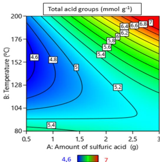
Fig. 2 Response surface obtained in the optimization process of sulfonated carbons through carbonization and *in situ* sulfonation. Effect of temperature and  $\text{H}_2\text{SO}_4$  quantity on total acidic groups quantification.
