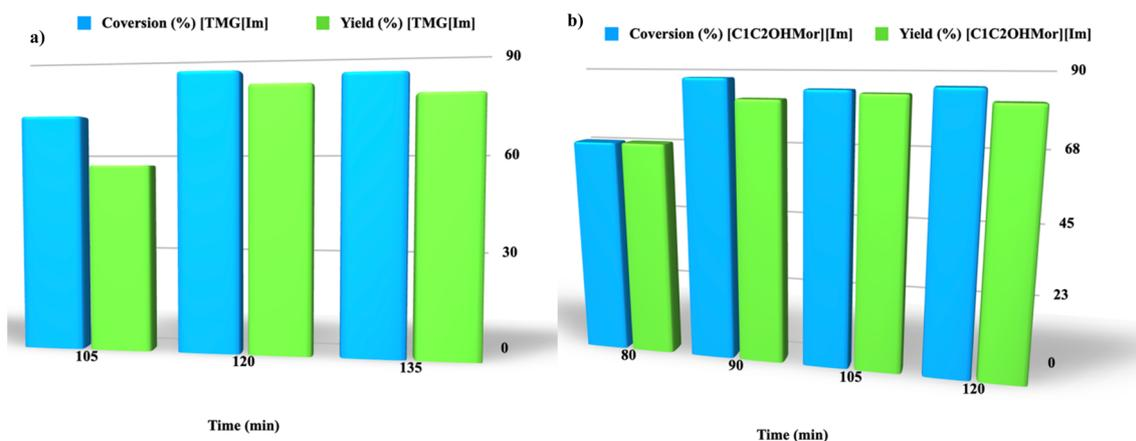
Fig. 3 Conversion and yield values for the methanolysis of BPA-PC, under US irradiation (50 W, 250 kHz) at 30 °C, as a function of time: (a) in the presence of [TMG][Im]; (b) in the presence of [C<sub>1</sub>C<sub>2</sub>OHMor][Im] ( $n_c/n_{RU} = 1/12$ ;  $m_{2\text{-MeTHF}}/m_{\text{MeOH}} = 3$ ). Conversion and yield values were reproducible within  $\pm 3\%$ .
