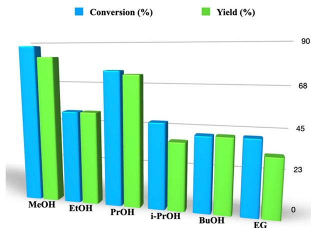
Fig. 5 Conversion and yield values for the alcoholysis of BPA-PC, under US irradiation (50 W, 250 kHz) at 30 °C, in the presence of different nucleophiles ( $n_c/n_{\text{RU}} = 1/12$ ;  $m_{2-\text{MeTHF}}/m_{\text{MeOH}} = 3$ ). Conversion and yield values were reproducible within  $\pm 3\%$ .
