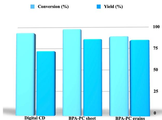
Fig. 8 Conversion and yield values collected for the methanolysis of a digital CD, BPA-PC sheet, and BPA-PC grains, using [C<sub>1</sub>C<sub>2</sub>OHHMor][Im] ( $n_c/n_{RU} = 1/12$ ;  $m_{2-MeTHF}/m_{MeOH} = 3$ ) as the catalyst, under US irradiation (50 W, 250 kHz) at 30  $^{\circ}$ C for 90 min. Conversion and yield values were reproducible within  $\pm 3\%$ .
