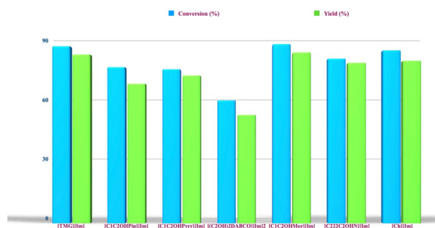
Fig. 1 Conversion and yield values for the methanolysis of BPA-PC, under US irradiation (50 W, 250 kHz) at 30 °C for 120 minutes, as a function of the nature of different catalysts ( n_c/n_{RU} = 1/12 ; m_{2-MeTHF}/m_{MeOH} = 3 ). Conversion and yield values were reproducible within \pm 3\% . Values for [Ch][Im] are taken from ref. 33.
