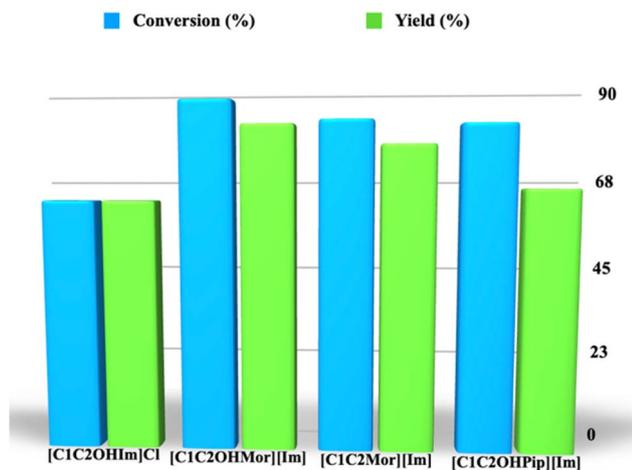
Fig. 4 Conversion and yield values for the methanolysis of BPA-PC, under US irradiation (50 W, 250 kHz) at 30 °C, in the presence of different catalysts ( $n_c/n_{\text{RU}} = 1/12$ ;  $m_{2\text{-MeTHF}}/m_{\text{MeOH}} = 3$ ). Conversion and yield values were reproducible within  $\pm 3\%$ .
