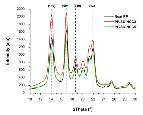
XRD diffractograms of neat PP and the PP/SD-NCC3 and PP/SD-NCC5 bionanocomposites
