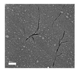
Fig. 3 TEM images of (a) wet NCC (W-NCC) and (b) spray-dried NCC (SD-NCC) at 100 00× magnification.
