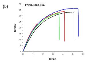
Fig. 8 Stress—Strain curves for PP/SD-NCC5 from (a) one-step and (b) two-step compounding.
