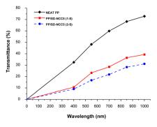
Fig. 10 Optical properties of neat PP and PP/SD-NCC bionano-composites after one-step and two-step compounding.
