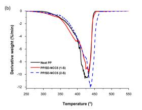
Fig. 11 (a) TGA and (b) DTG thermographs of neat PP and PP/SD-NCC bionanocomposites after one-step and two-step compounding.
