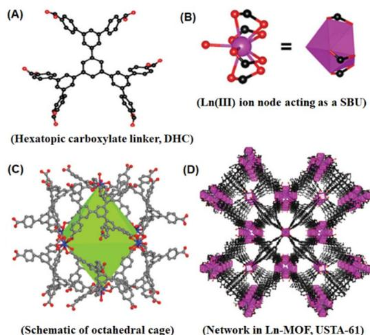
**Fig. 15** Schematics of (A) hexatopic carboxylate linker DHC, (B)  $\text{Ln(III)}$  ion node as SBU involving DHC ligands, (C) octahedral cage involving six  $\text{Ln(III)}$  ion nodes and eight organic linkers, and (D) construction of the overall mesoporous network for the USTA-61 materials. The figure is redrawn from ref. 4 & 146 with permission from the Royal Society of Chemistry.
