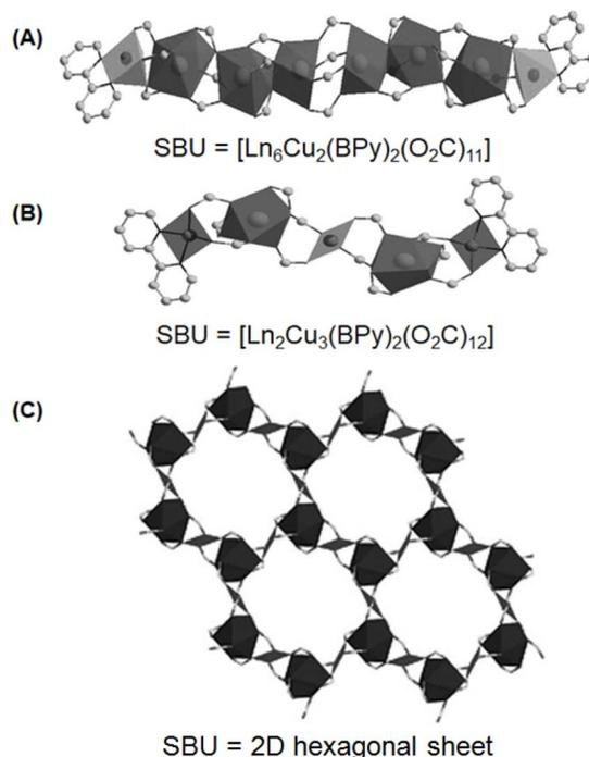
Fig. 11 Two different rod-shaped SBUs with constructions as (A)  $[\text{Ln}_6\text{Cu}_2(\text{BPy})_2(\text{O}_2\text{C})_{11}]$ , and (B)  $[\text{Ln}_2\text{Cu}_3(\text{BPy})_2(\text{O}_2\text{C})_{12}]$ , and (C) the 2D hexagonal sheet, as obtained by using IP and BPy as the O-donor and N-donor ligands, respectively, for the synthesis of Ln-TM-MOF systems involving Ln(III) (Ln = Er, Y and Eu) and Cu(II) ions. The figure is redrawn from ref. 136 with permission from Wiley Inter Science.
