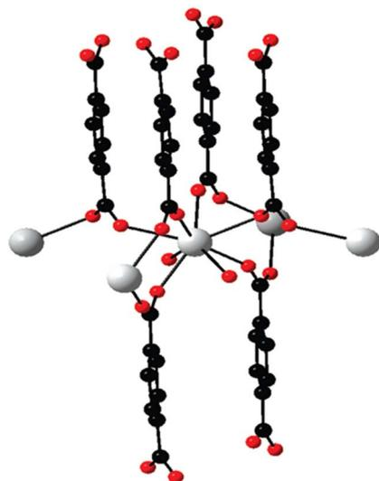
Fig. 9 Projection of an extended asymmetric unit of  $[\text{Tb}_2(\text{BDC})_3(\text{H}_2\text{O})_4]_n$ . Color codes: Ln (white); O (red); and C (black). Reproduced from ref. 130 with permission from the American Chemical Society.
