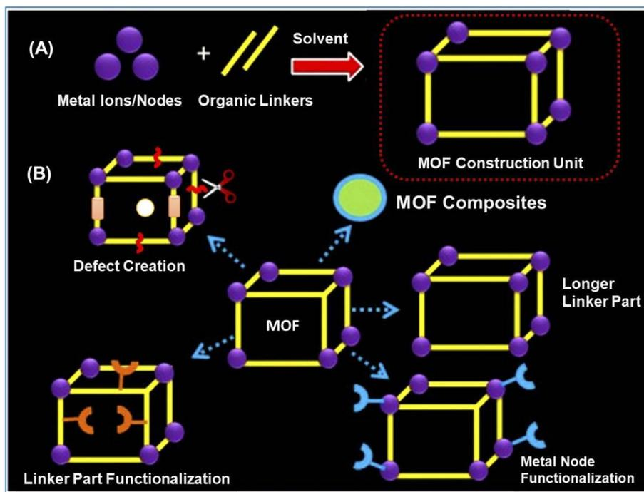
Fig. 2 (A) General scheme for the synthesis of MOF materials *via* the bottom-up approach involving the direct reaction of metal nodes and organic linkers under suitable reaction conditions. (B) Different strategies reported for boosting the performance of MOF materials by their suitable functionalizations.
