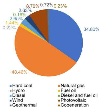
Fig. 7 Northern Chilean electrical grid fuel mix.<sup>45</sup>
