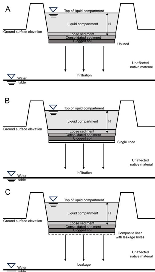
Fig. 6 Three types of surface impoundments considered. (A) Unlined. (B) Single lined. (C) Composite liner with leakage holes.<sup>62</sup>
