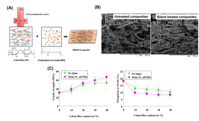
Fig. 8 (A) Schematic representation of the fabrication of silane-treated PBS/cotton fiber composites; (B) morphology of untreated and silanetreated composites and (C) mechanical properties of PBS/cotton fiber composites with and without silane treatment. Reproduced from ref. 158, MDPI, 2013, Open Access
