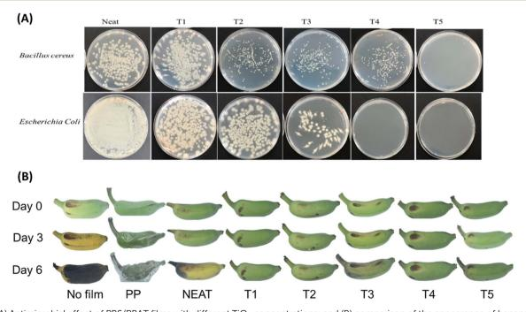
Fig. 12 (A) Antimicrobial effect of PBS/PBAT films with different  $TiO_2$  concentrations; and (B) comparison of the appearance of bananas in their natural state (no film) to those wrapped in PP and PBAT/PBS films with varying  $TiO_2$  levels [neat (0.9%), (T2) 1.8%, (T3) 2.7%, (T4) 3.6%, and (T5) 4.5%]. Reproduced with permission from ref. 201, Elsevier, 2023.
