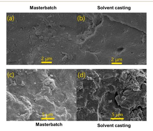
Fig. 10 Morphology of PBS/NFC (a and c) masterbatch and (b and d) solvent cast films. The masterbatch film exhibited a uniform film surface with fewer defects and voids compared to solvent-cast films. Reproduced with permission from ref. 167, Elsevier, 2021.
