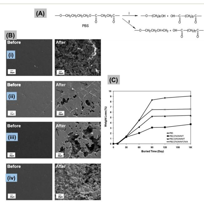
Fig. 14 (A) Mechanism of PBS degradation; (B) SEM micrographs of (i) PBS, (ii) PBS/2% MMT, (iii) PBS/10% MMT and (iv) compatibilized PBS nanocomposites; and (C) weight loss of PBS and its nanocomposites; OMMT: organo-montmorillonite. Reproduced with permission from ref. 245, Elsevier, 2012.
