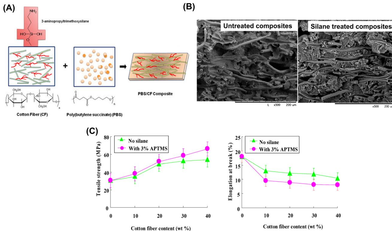
Fig. 8 (A) Schematic representation of the fabrication of silane-treated PBS/cotton fiber composites; (B) morphology of untreated and silane-treated composites and (C) mechanical properties of PBS/cotton fiber composites with and without silane treatment. Reproduced from ref. 158, MDPI, 2013, Open Access.
