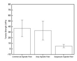
Fig. 9 Tensile strength of calcium alginate fibres from different sources.
