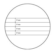
Fig. 4 The preparation of the paper specimen for tensile strength measurement.
