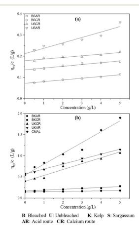
Fig. 6 Specific viscosity  $(\eta_{\rm sp})$  of sodium alginate samples in 0.1 M NaCl from (a) *S. polycystum* and (b) *L. japonica*.
