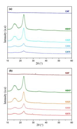
Fig. 15 XRD patterns of the calcium alginate fibres, HBKP, and paper composites containing (a) commercial alginate fibres (CA) and (b) kelp alginate fibres (KA).
