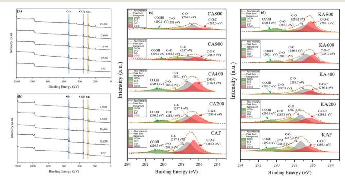
Fig. 16 XPS spectra of residual calcium alginate after thermal treatment at 200, 400, 600, and 800  $^{\circ}$ C in the wide scan of (a) the commercial alginate fibre sample and (b) the kelp alginate fibre sample, and high-resolution  $C_{1s}$  spectra of (c) commercial alginate fibres and (d) kelp alginate fibres.
