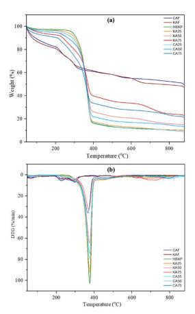
Fig. 13 (a) Thermogravimetric (TG) and (b) DTG curves of calcium alginate fibres and paper composites.
