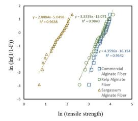
Fig. 8 Weibull plots for different types of calcium alginate fibre sources.
