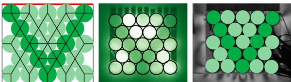
**Evolution of adaptive force chains in reconfigurable granular metamaterials**
