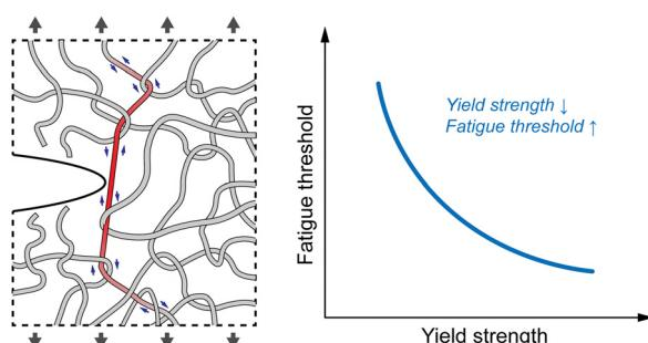
**How does a polymer glass resist fatigue crack growth?**
