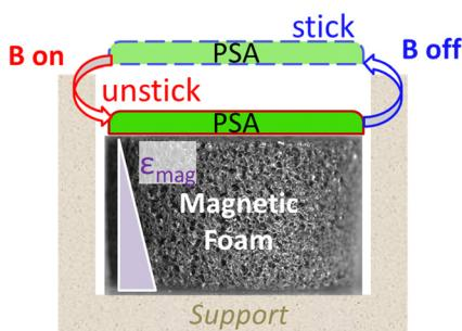
**"Magnetic marshmallows" for soft robotics: magneto-mechanical characterization and application in switchable adhesion structures**
