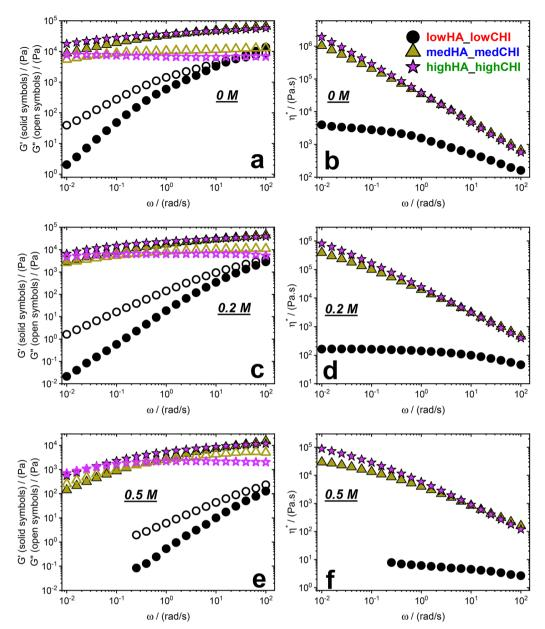
Fig. 3 Linear viscoelasticity of symmetrical pairs. Storage modulus G' (closed symbols), loss modulus G' (open symbols), and complex viscosity  $\eta^*$ , as a function of oscillation frequency  $\omega$  for the symmetric  $M_w$  samples across three different salt concentrations (a) and (b) 0 M, (c) and (d) 0.2 M, and (e) and (f) 0.5 M. The labels are color-coded for ease of perusal. The colors red, dark blue, and green indicate low, medium, and high  $M_w$ , respectively.
