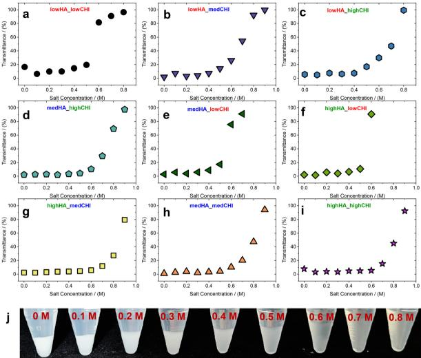
Fig. 2 UV-Vis spectroscopy. (a)–(i) Evolution of the transmittance determined by UV-vis spectroscopy upon the addition of CHI solutions (of varying M<sub>W</sub>) to HA solutions (of varying  $M_w$ ) as a function of NaCl concentration. The pairs of polyanion-polycation are labeled in their respective plots. (j) Images of complex coacervates obtained from HA-CHI (lowHA\_medCHI) samples of varying salt concentrations in the range 0.0-0.8 M NaCl, after centrifugation.
