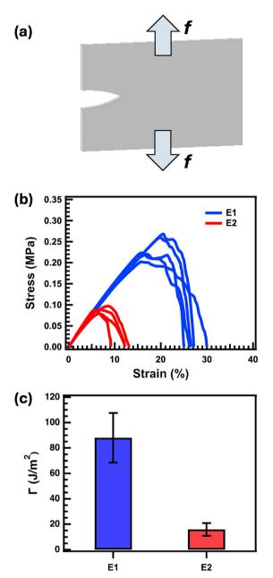
Fig. 5 The tear test according to the Rivalan-Thomas method on (a) notched elastomer samples in pure shear geometry, yielding (b) uniaxial extension stress-strain curves which was used to calculate (c) tearing energies for E1 and E2
