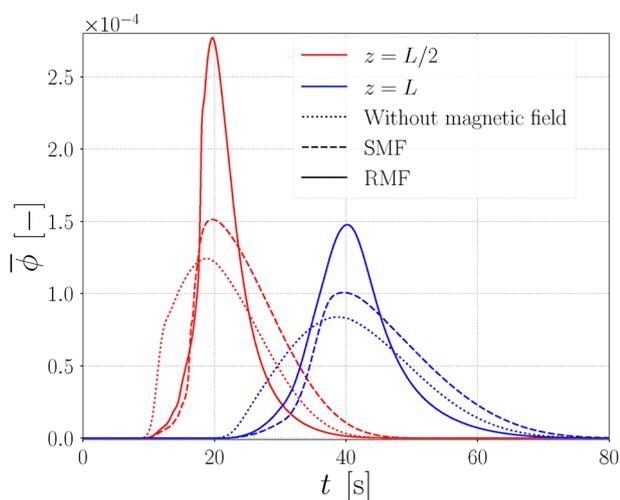
**Fig. 8** Cross-sectionally averaged MNP concentration signals at  $z = L/2$  and  $z = L$  for no field, SMF, and RMF at  $f_0 = 100$  kHz, showing enhanced variance reduction under RMF. Parameters:  $v_0 = 0.25$  mm  $s^{-1}$  ( $Pe \approx 1145$ ,  $Re \approx 0.05$ );  $H_0 = 14.713$  kA  $m^{-1}$  ( $\alpha = 1$ ); injected concentration  $\phi_0 = 5 \times 10^{-5}$ ; particle diameter  $D_p = 10$  nm; domain magnetization  $M_d = 425$  kA  $m^{-1}$ .
