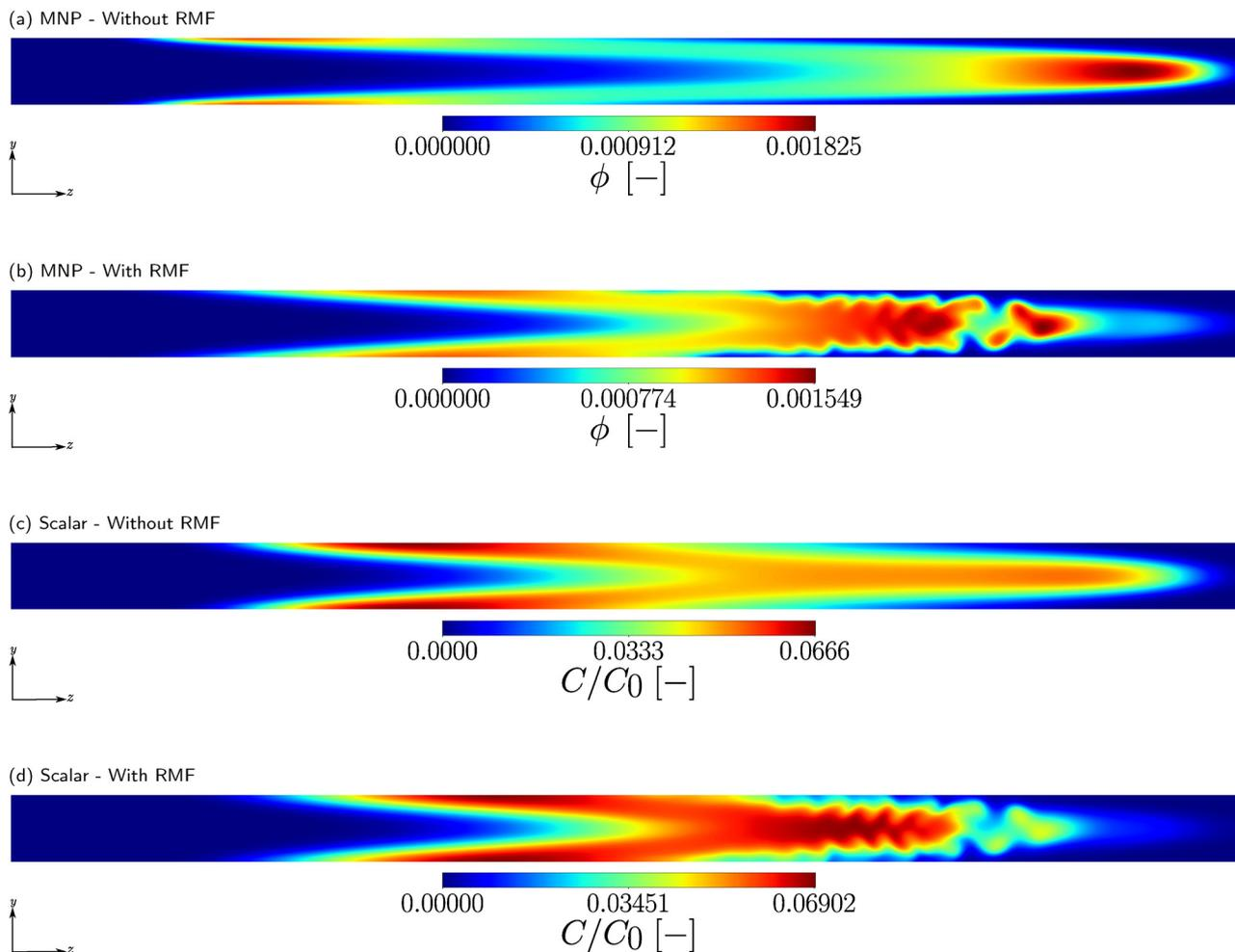
**Fig. 14** Comparison of passive scalar and MNP concentration contours at  $t = 2$  s for simultaneous pulse injection with  $\phi_0 = 5 \times 10^{-4}$ ,  $f_0 = 500$  kHz, and space time  $\bar{t} = 4$  s: (a) and (c) without RMF, (b) and (d) with RMF. Parameters:  $v_0 = 0.25$  mm s $^{-1}$  ( $Pe \approx 1145$ ,  $Re \approx 0.05$ );  $H_0 = 14.713$  kA m $^{-1}$  ( $\alpha = 1$ ); particle diameter  $D_p = 10$  nm; domain magnetization  $M_d = 425$  kA m $^{-1}$ .
