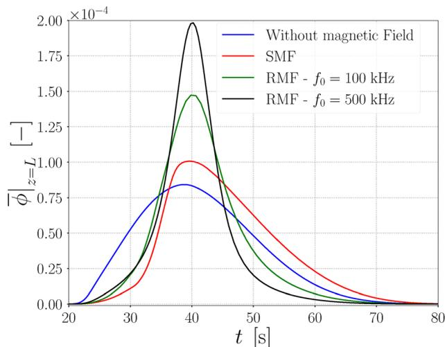
**Fig. 13** Effect of RMF frequency on outlet MNP concentration signals for  $\phi_0 = 5 \times 10^{-5}$ . Parameters:  $v_0 = 0.25 \text{ mm s}^{-1}$  ( $Pe \approx 1145$ ,  $Re \approx 0.05$ );  $H_0 = 14.713 \text{ kA m}^{-1}$  ( $\alpha = 1$ ); particle diameter  $D_p = 10 \text{ nm}$ ; domain magnetization  $M_d = 425 \text{ kA m}^{-1}$ .
