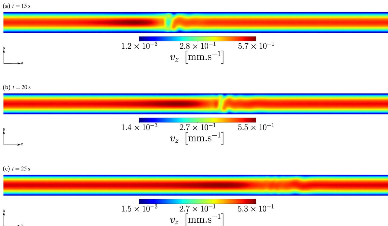
**Fig. 11** Contour plots of the axial velocity component  $v_z$  in the  $yz$ -plane at  $x = 0$ , shown at (a)  $t = 15$  s, (b)  $t = 20$ , and (c)  $t = 25$  s under an RMF ( $f_0 = 100$  kHz). Parameters:  $v_0 = 0.25$  mm s $^{-1}$  ( $Pe \approx 1145$ ,  $Re \approx 0.05$ );  $H_0 = 14.713$  kA m $^{-1}$  ( $\alpha = 1$ ); injected concentration  $\phi_0 = 5 \times 10^{-5}$ ; particle diameter  $D_p = 10$  nm; domain magnetization  $M_d = 425$  kA m $^{-1}$ .
