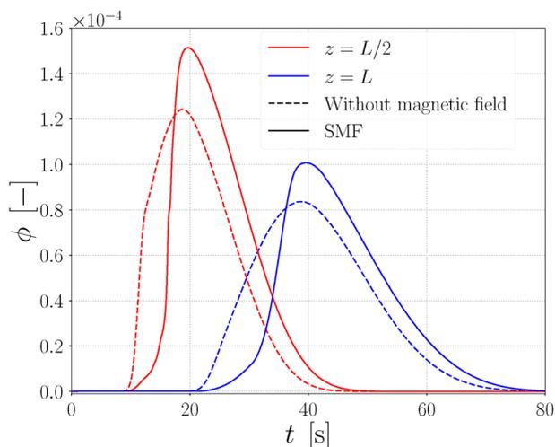
**Fig. 2** Temporal evolution of the cross-sectionally averaged MNP concentration at  $z = L/2$  and  $z = L$  for an inlet velocity  $v_0 = 0.25 \text{ mm s}^{-1}$  ( $\text{Pe} \approx 1145$ ,  $\text{Re} \approx 0.05$ ), comparing the cases without a magnetic field and with an SMF ( $\alpha = 1$ ,  $H_0 = 14.713 \text{ kA m}^{-1}$ ). The injected concentration is  $\phi_0 = 5 \times 10^{-5}$ ; particle diameter  $D_p = 10 \text{ nm}$ ; domain magnetization  $M_d = 425 \text{ kA m}^{-1}$ .
