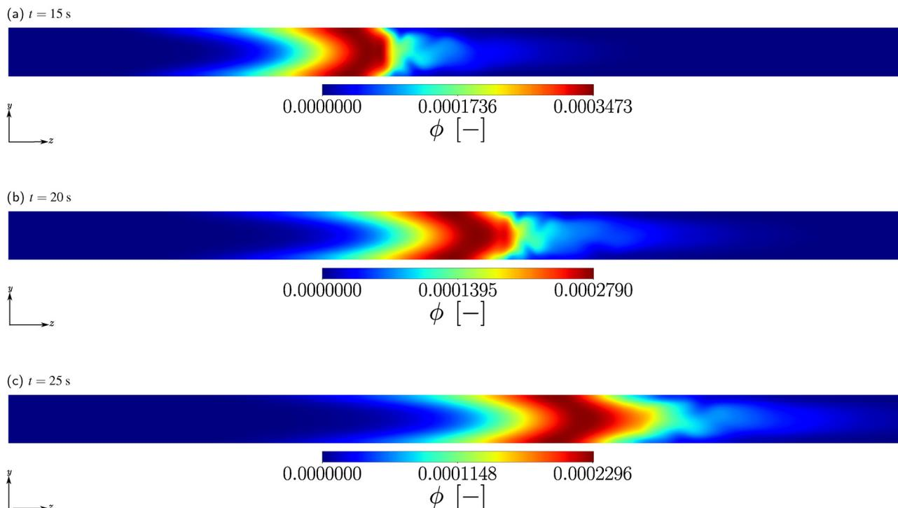
**Fig. 10** MNP concentration field in the  $yz$ -plane under an RMF at  $f_0 = 100$  kHz at (a)  $t = 15$  s, (b)  $t = 20$  s, and (c)  $t = 25$  s. Parameters:  $v_0 = 0.25$  mm s $^{-1}$  ( $Pe \approx 1145$ ,  $Re \approx 0.05$ );  $H_0 = 14.713$  kA m $^{-1}$  ( $\alpha = 1$ ); injected concentration  $\phi_0 = 5 \times 10^{-5}$ ; particle diameter  $D_p = 10$  nm; domain magnetization  $M_d = 425$  kA m $^{-1}$ .
