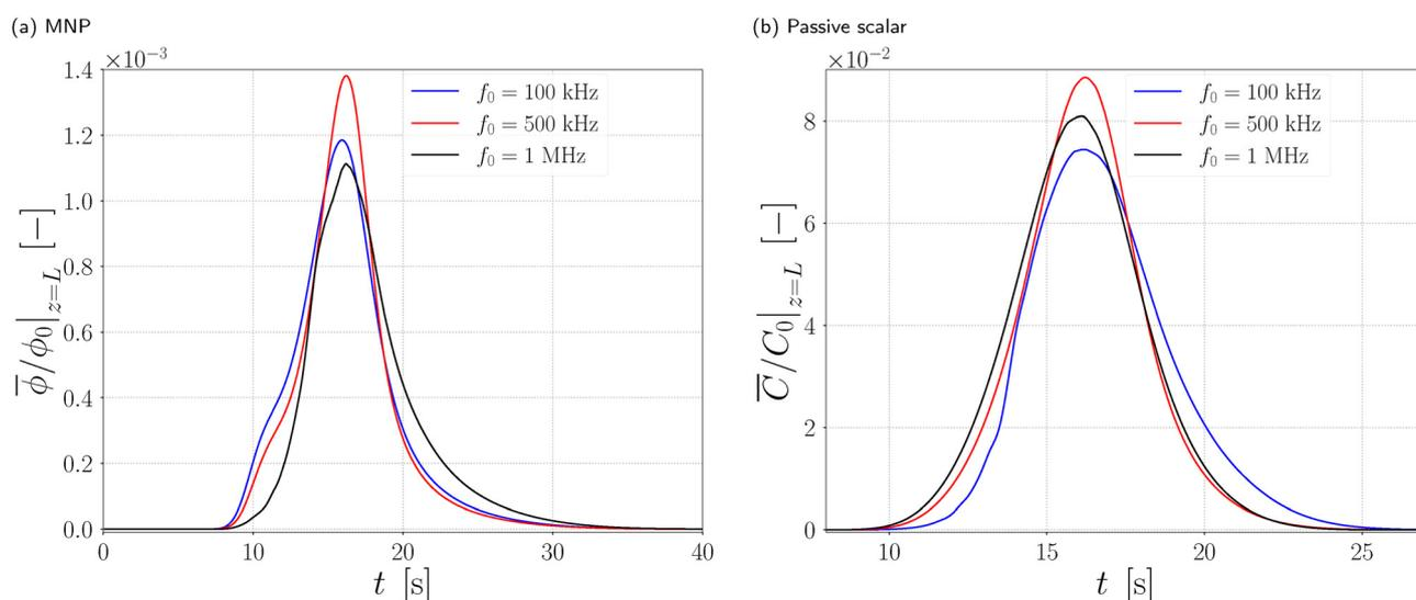
Fig. 18 RMF frequency dependence of outlet concentration signals at  $\bar{t} = 16$  s for  $\phi_0 = 5 \times 10^{-4}$ : (a) MNPs and (b) passive scalar, showing resonance-like enhancement of mixing at  $f_0 = 500$  kHz. Parameters:  $v_0 = 0.25$  mm  $s^{-1}$  ( $Pe \approx 1145$ ,  $Re \approx 0.05$ );  $H_0 = 14.713$  kA  $m^{-1}$  ( $\alpha = 1$ ); particle diameter  $D_p = 10$  nm; domain magnetization  $M_d = 425$  kA  $m^{-1}$ .
