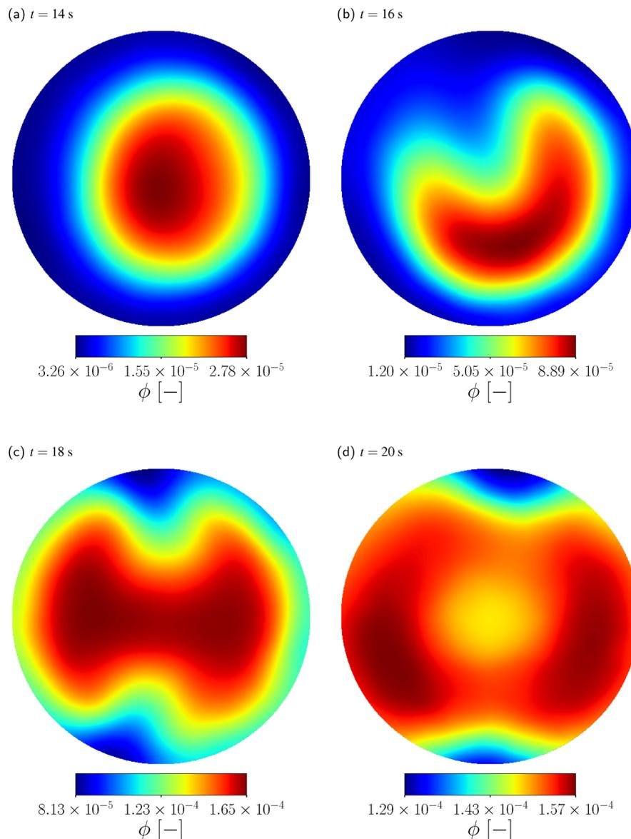
Fig. 4 Cross-sectional MNP concentration contours at  $z = L/2$  and times (a)  $t = 14$  s, (b)  $t = 16$  s, (c)  $t = 18$  s, and (d)  $t = 20$  s, showing the loss of symmetry under an SMF ( $\alpha = 1$ ,  $H_0 = 14.713$  kA  $m^{-1}$ ). Parameters:  $v_0 = 0.25$  mm  $s^{-1}$  ( $Pe \approx 1145$ ,  $Re \approx 0.05$ ); injected concentration  $\phi_0 = 5 \times 10^{-5}$ ; particle diameter  $D_p = 10$  nm; domain magnetization  $M_d = 425$  kA  $m^{-1}$ .
