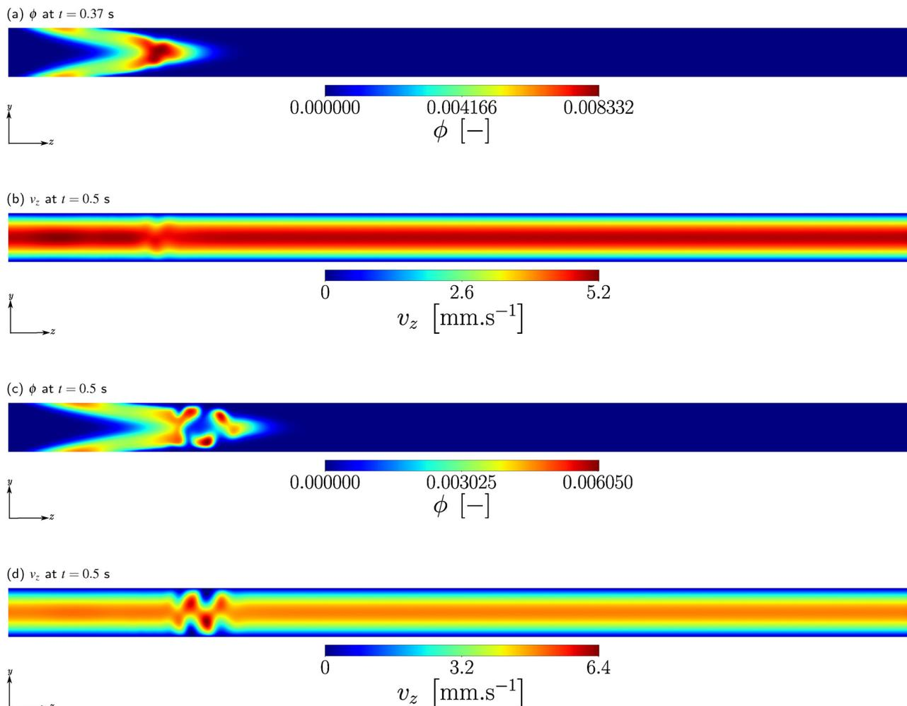
Fig. 15 Contours of MNP concentration (a) and (c) and axial velocity (b) and (d) at  $t = 0.37$  s and  $t = 0.5$  s for  $\bar{t} = 4$  s,  $Pe \approx 1.1 \times 10^4$ , and  $\phi_0 = 5 \times 10^{-4}$ . Parameters:  $v_0 = 0.25$  mm s $^{-1}$  ( $Re \approx 0.05$ );  $H_0 = 14.713$  kA m $^{-1}$  ( $\alpha = 1$ ); particle diameter  $D_p = 10$  nm; domain magnetization  $M_d = 425$  kA m $^{-1}$ .
