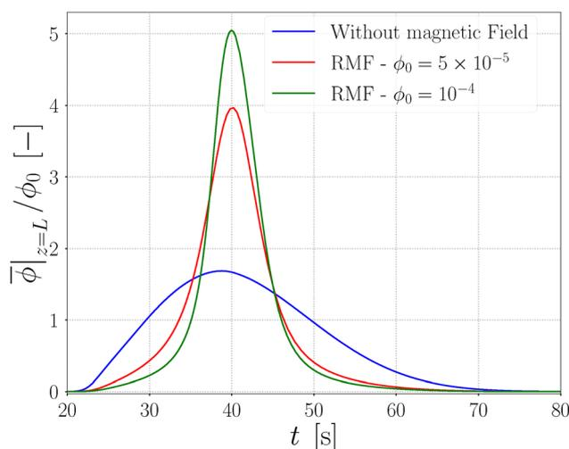
**Fig. 12** Effect of injected MNP concentration on outlet signals under an RMF at  $f_0 = 100$  kHz, compared with the no-field case. Parameters:  $v_0 = 0.25$  mm s $^{-1}$  ( $Pe \approx 1145$ ,  $Re \approx 0.05$ );  $H_0 = 14.713$  kA m $^{-1}$  ( $\alpha = 1$ ); injected concentrations  $\phi_0 = 5 \times 10^{-5}$  and other values as indicated; particle diameter  $D_p = 10$  nm; domain magnetization  $M_d = 425$  kA m $^{-1}$ .
