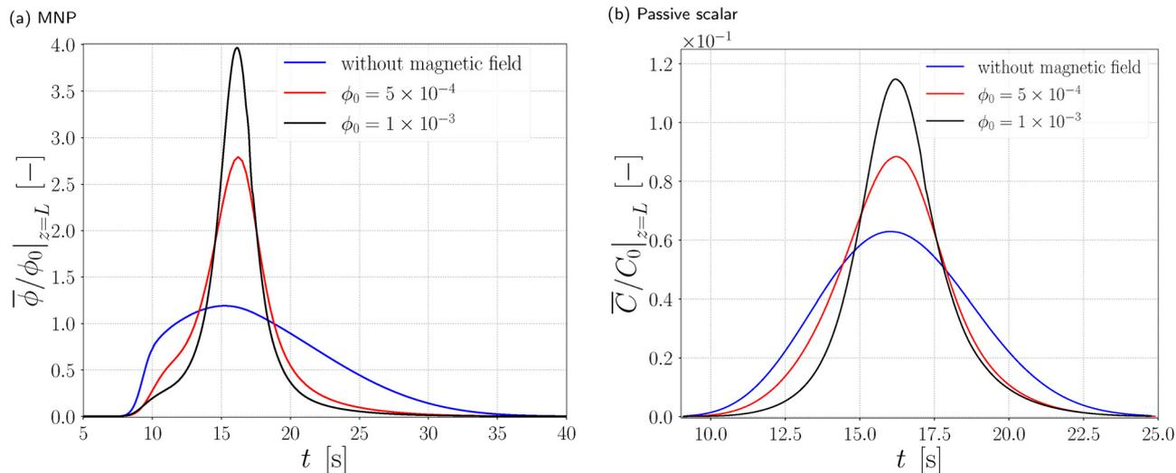
Fig. 17 Outlet concentration signal at  $\bar{t} = 16$  s for  $\phi_0 = 5 \times 10^{-4}$  under an RMF at  $f_0 = 500$  kHz: (a) MNPs and (b) passive scalar. Parameters:  $v_0 = 0.25$  mm  $s^{-1}$  ( $Pe \approx 1145$ ,  $Re \approx 0.05$ );  $H_0 = 14.713$  kA  $m^{-1}$  ( $\alpha = 1$ ); particle diameter  $D_p = 10$  nm; domain magnetization  $M_d = 425$  kA  $m^{-1}$ .
