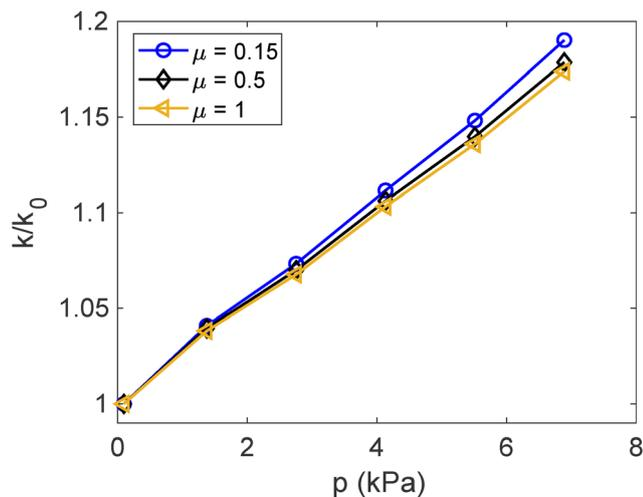
Fig. 9 The normalized compressive stiffness  $k/k_0$  from ABAQUS simulations of type I particles with a ratio of the fillet radius to the wall thickness  $r/t = 2$  plotted versus the inflation pressure  $p$  (in kPa). The friction coefficient between the Ecoflex particles and steel walls is varied over the range  $0.15 \leq \mu \leq 1$ .
