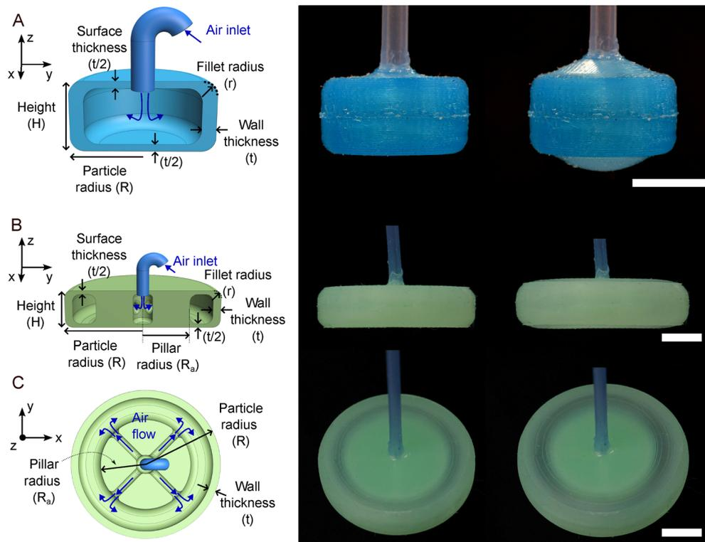
**Fig. 1** Schematic of the two types of particles (left) with images in the uninflated (middle) and inflated (right) states. Side views of (A) type I and (B) type II particles. (C) Top view of a type II particle. The type I and II particles have been inflated to  $\sim 3.4$  kPa and  $\sim 8.6$  kPa, respectively. All scale bars correspond to 10 mm.
