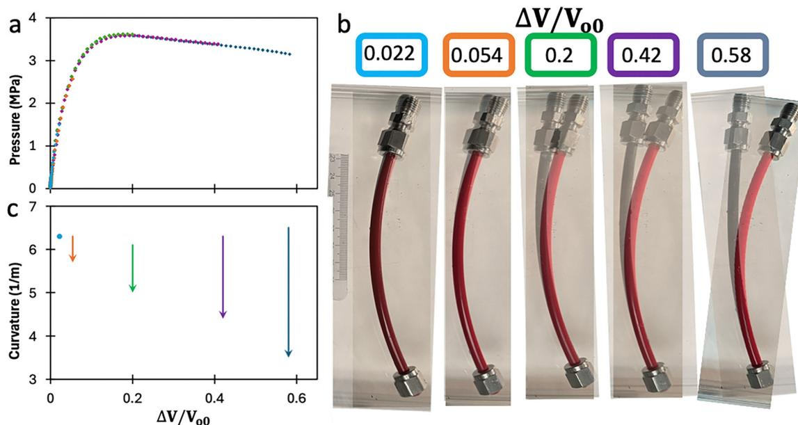
Fig. 6 (a) Pressure–volume curves for five tube specimens inflated to various pressures. (b) Each image shows an overlay of the initial shape of the tube before inflation in red and after deflation in gray. (c) Initial and final curvature after deflation, measured along the inner perimeter, for each sample. Each arrow is drawn to start at the initial curvature and end at the final curvature after deflating the tube.
