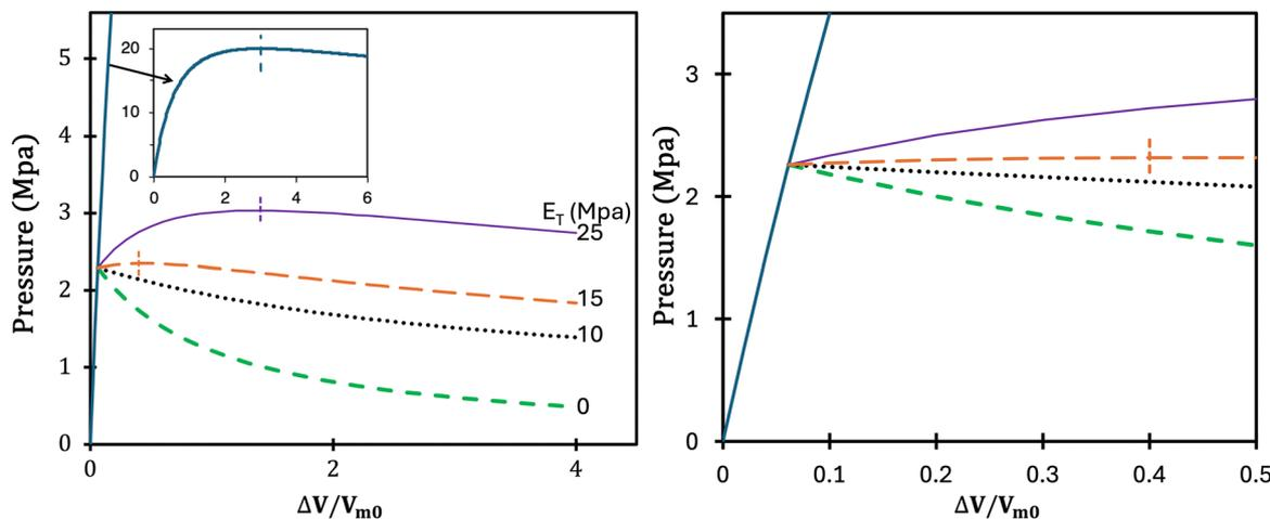
Fig. 7 Pressure–volume behavior predicted by the approximate thin shell model for various levels of tangential modulus parameter  $E_T$ . Right graph magnifies the behavior at small volume. Blue line is linearly elastic, eqn (10), which is shown over a larger range of pressures in the inset to the left graph. Small vertical lines indicate location of the maximum.
