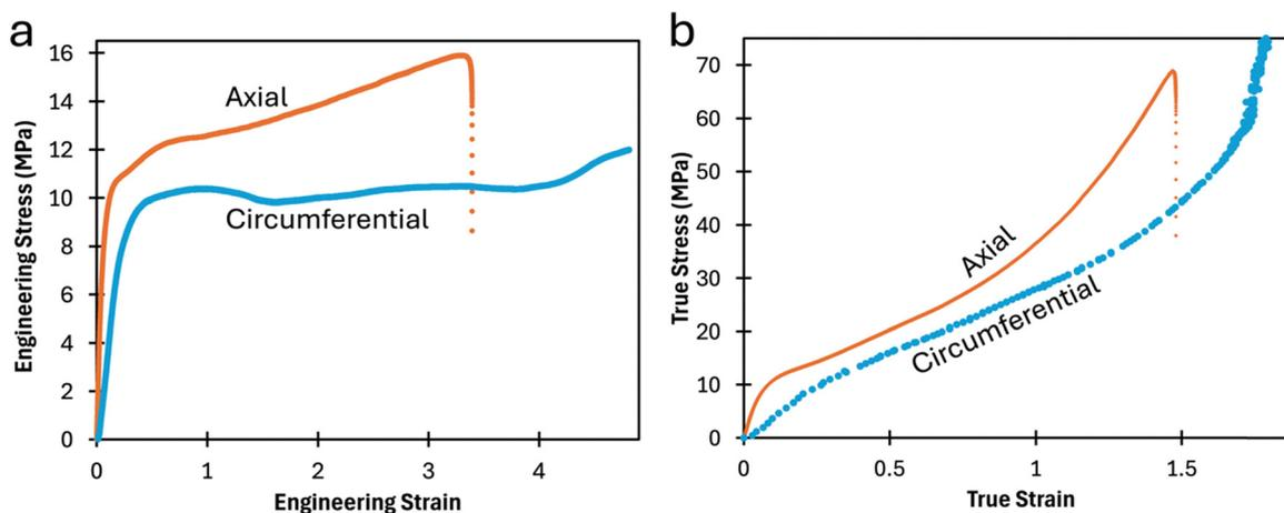
Fig. 3 (a) Engineering stress *vs.* engineering strain curves for an axially-stretched sample in orange and a circumferentially-stretched sample in blue. (b) Same data as a, but plotted with true values of stress and strain. The circumferential data at small strains are unreliable because the samples do not start from a stress-free state, see text and Section S2.
