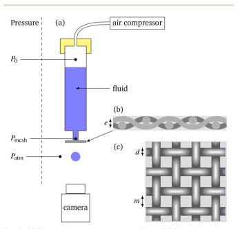
Fig. 1 (a) Quasi-static experimental setup. (b) and (c) Side-view and topview diagrams, respectively, of the woven polyamide meshes (diagrams provided by the manufacturer). Definition of key dimensions: pore size m, fiber diameter d, and mesh thickness e
