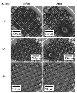
Fig. 9 Snapshots from experimental videos obtained with mesh 5 and three different yield stresses (O Pa, 4.4 Pa, 86 Pa). Snapshots referenced as 'before' are taken just before the start of the flow and those referenced as 'after' are taken just after. The comparison of the reflection patterns between two snapshots (before/after) gives information about the existence or not of fluid retraction
