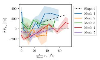
Fig. 6 Yield-stress contribution to the penetration pressure  $\Delta P_{\sigma_{ij}}$  as a function of the rescaled yield stress ( $e/m_{\rm real}$ ) $\sigma_{y_i}$  for the five mesh géometries. The dotted line corresponds to  $\beta$  = 4 in eqn (3). Each point represents the average value for a set of parameters ( $\sigma_y$ , m, e) over 2 to 10 experiments. The lighter-colored areas indicate the corresponding standard deviations.
