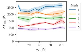
Fig. 5 Penetration pressure  $\Delta P_{\rm pen}$  as a function of yield stress  $\sigma_{\rm y}$ , for the five meshes used. Each point represents the average value for a set of parameters ( $\sigma_{v}$ , m, e) over 2 to 10 experiments. The lighter-colored areas indicating the corresponding standard deviations.
