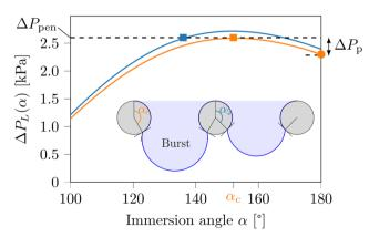
Fig. 8 Main: Laplace pressure as a function of the immersion angle for two pores differing in size or wetting properties. One of them (orange curve) is characterized by a smallest capillary pressure. Inset: Illustration of meniscus advancement in two pores with different capillary pressures. The liquid goes through the pore with the smallest maximum pressure.
