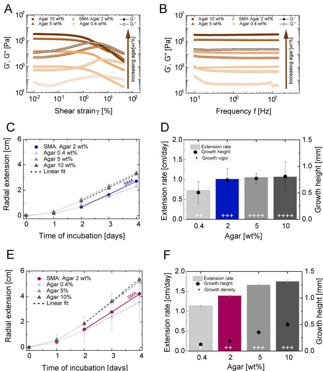
Fig. 5 Influence of agar gel strength on mycelium growth. Development of the storage modulus  $G'$  and loss  $G''$  moduli of SMA with 0.4, 2, 5, and 10 wt% agar upon applied (A) strain and (B) frequency. (C) and (E) show the radial extension of *P. ostreatus* and *P. djamora* over time as a function of gel strength. (D) and (F) show the extension rate in comparison to growth height and mycelium density. Values are expressed as mean  $\pm$  standard deviation ( $n = 3$ ).
