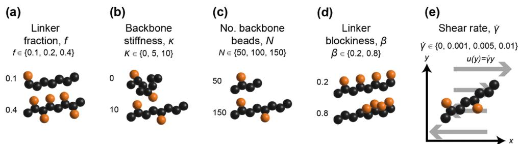
**Fig. 1** Overview of precursor chain parameters studied. (a) Linker fraction  $f$  is the ratio of reactive linker beads to backbone beads. (b) Stiffness  $\kappa$  indicates the tendency for the chain to resist bending. (c) Number of backbone beads  $N$ . (d) Blockiness  $\beta$  quantifies reactive bead clustering. (e) Shear rate  $\dot{\gamma}$ . Values indicated in each panel are the lower and upper limits of the parameter range in reduced units.
