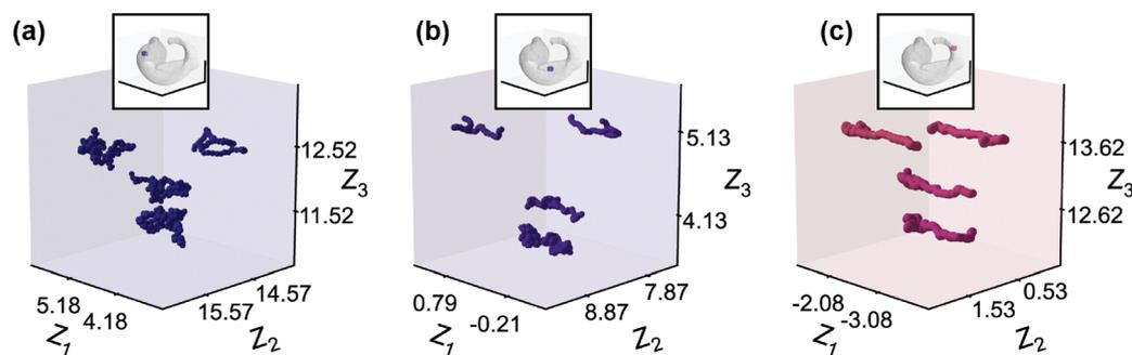
**Fig. 3** Representative regions of the embedding space and corresponding SCNP morphologies. (a) Globular chains at low  $Z_1$ . (b) Semi-elongated structures at intermediate  $Z_1$ . (c) Elongated rod-like morphologies at high  $Z_1$ . Insets indicate the location of each zoomed-in region within the embedding space.
