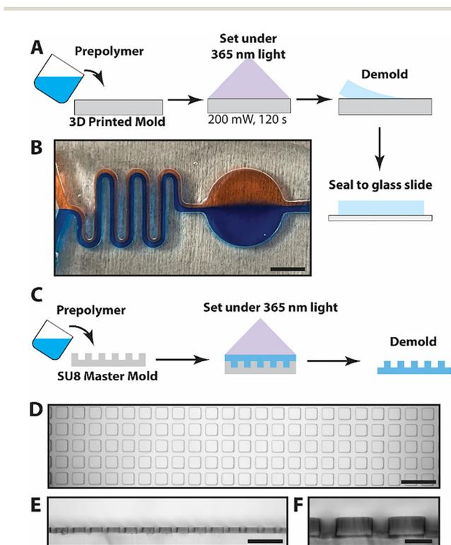
Fig. 3 (A) Schematic of bulk UV-set replica molding workflow. (B) Optical image of replica molded UV-set PDMS microfluidic device under 1 mL min<sup>-1</sup> flow conditions. The scale bar is 5 mm. (C) Schematic of soft lithography UV-set workflow. (D) Microscope image of UV-set PDMS molded from an SU-8 Master Mold with 50 μm squares. The scale bar is 200 μm. (E) Optical cross section of (D) with a 200 μm scale bar. (F) A closer cross section of (D). The scale bar is 50 μm.
