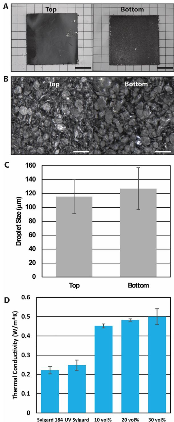
**Fig. 4** (A) Optical image of the top and bottom of the liquid metal composite, scale bars are 1 cm. (B) Microscope images of the top and bottom of a 20% filled sample, scale bars are 250  $\mu\text{m}$ . (C) Particle size analysis of the droplets in (B) calculated with ImageJ. (D) Thermal conductivity as a function of sample composition. Error bars represent the standard deviation for 3 samples and 100 particles respectively.
