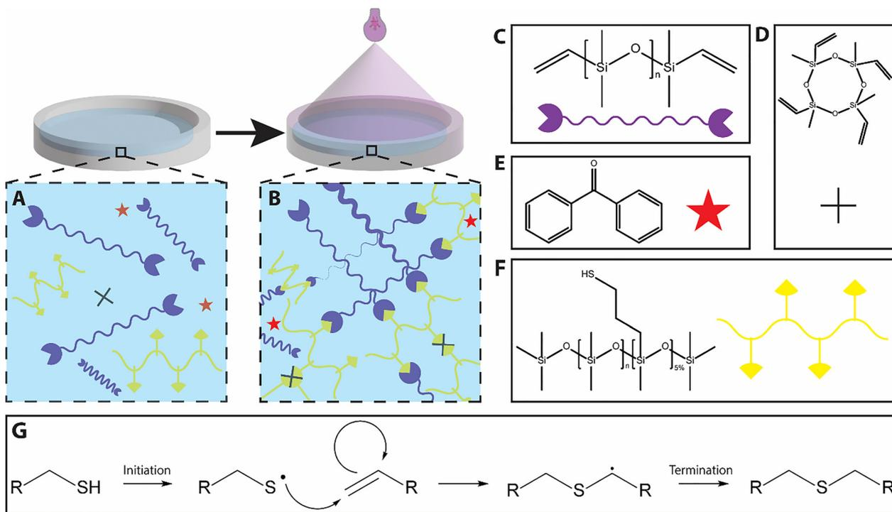
**Fig. 1** Curing scheme of UV-set PDMS. (A) Prepolymer solution. (B) Cured UV-set PDMS. Chemical structures of the components of UV-set PDMS: (C) vPDMS, (D) vD4, (E) benzophenone, and (F) MPPDMS. (G) The thiol-ene reaction expected in our system.
