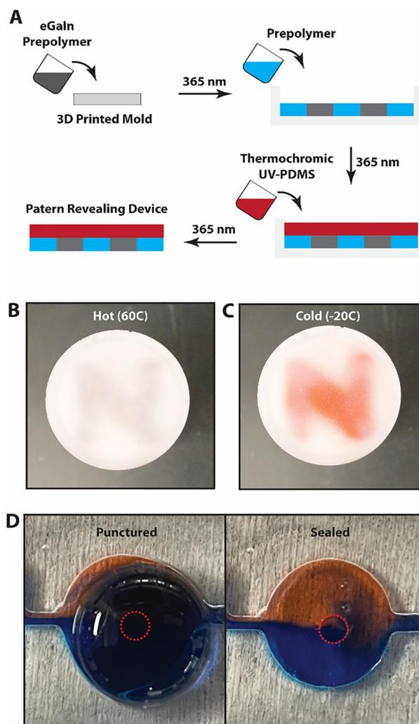
**Fig. 5** (A) Schematic of thermal pattern revealing device fabrication. Optical images of the thermal pattern revealing device when warmed to 60  $^{\circ}\text{C}$  (B) and when placed on a  $-20^{\circ}\text{C}$  cold sink (C). (D) UV PDMS microfluidic device after puncturing with a 2.5 mm biopsy punch and subsequent rapid repair with UV PDMS. Red circles indicate the location of the punch.
