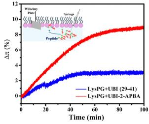
Fig. 6 Percentage change of surface pressure  $(\pi)$  of the Lys PG monolayer with time due to injection of UBI (29-41) (blue curve) and UBI-2-APBA (red curve) peptides in the subphase at an initial surface pressure of  $\sim$  20 mN m<sup>-1</sup>. The change is plotted relative to the change observed in pristine Lys PG. Inset: Schematic of the experiment showing the injected peptides diffusing to the lipid monolayer.
