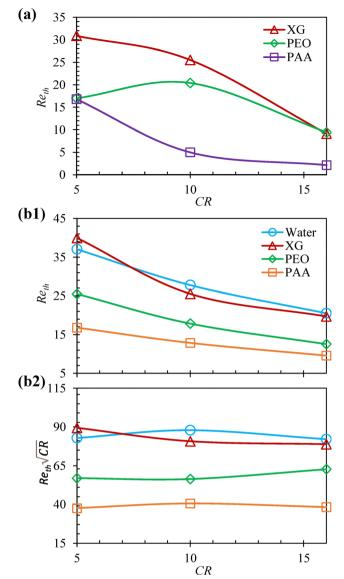
Fig. 9 Comparison of the threshold Reynolds number, Re<sub>th</sub>, for the onset of flow instability in the tested fluids through constriction microchannels with varying CR: (a) Re<sub>th</sub> in the contraction flow; (b1) Re<sub>th</sub> and (b2) Re<sub>th</sub>  $\sqrt{CR}$  in the expansion flow. All the lines are used to guide the eyes only.
