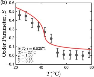
Fig. 4 Order parameter ( $S = \langle P_2 \rangle$ ) data obtained from Raman spectroscopy measurements for (a) 1× sample and (b) 1/8× sample. The red lines show the numerical fit to the data by solving eqn (16), with the relevant fitting parameters shown for each case.
