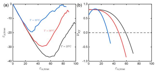
Fig. 10 (a) True strain  $(\varepsilon_y)$  in the y direction vs. true strain  $(\varepsilon_x)$  in the x direction for the 1× sample at strain rates of 0.5% min<sup>-1</sup> at T=23 °C (black), T=100 °C (b 30 °C (red), (c) T = 35 °C (blue). (b) Instantaneous x-y Poisson's ratio ( $\nu_{xy}$ ) vs. true strain ( $\epsilon_x$ ) in the x direction for the 1× sample at a strain rate of 0.5%  $min^{-1}$  at T = 23 °C (black), T = 30 °C (red), (c) T = 35 °C (blue).
