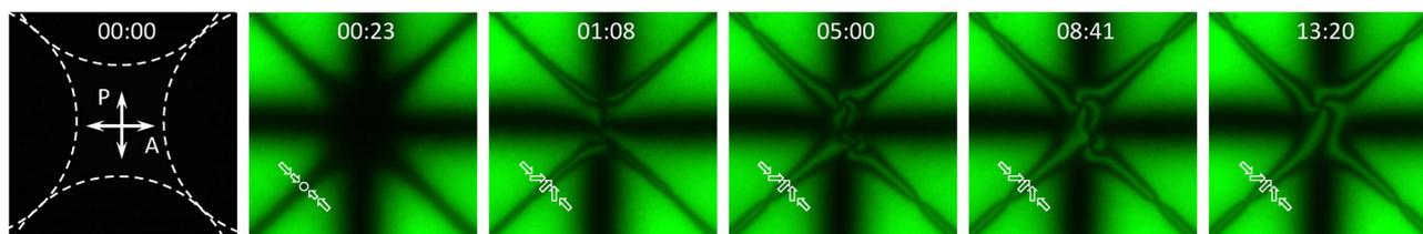
Fig. 4 Formation of transient textures in nematic slab seeded by the structured magnetic field obtained from a slightly asymmetric ( $b = 1.05a$ ) magnetic array and grown by the application of a uniform electric field. Each cross-polarized microscope image shows a 6 mm  $\times$  6 mm field of view. The timestamps are given in mm:ss format. The white arrows illustrate local Ising-like and Néel-like distributions of in-plane director orientation.
