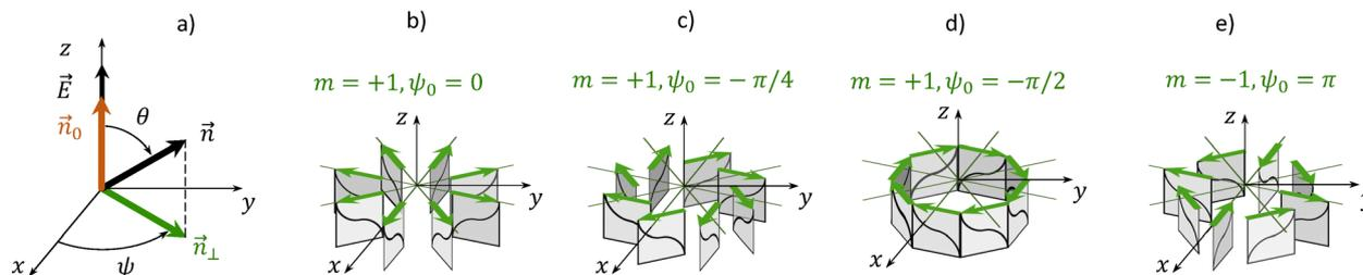
**Fig. 1** (a) Definition of the main vectors and angles. (b–e) Sketches of 3D structure of umbilics with  $m = \pm 1$  and different  $\psi_0$ . For each meridional cross-section oriented at an angle  $\phi$  from 0 to  $2\pi$  by step of  $\pi/4$ , the black solid line indicates the streamline of  $\vec{n}$  and the green arrow indicates its projection  $\vec{n}_\perp$  on the  $(x,y)$  plane.
