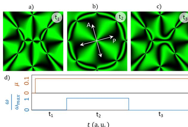
**Fig. 9** Numerical equivalent of cross polarized images of simulated topological textures for structured magnetic fields provided by the magnet configuration illustrated in Fig. 8 with  $A_{st} \approx 0.3$ . (a) before, (b) during and (c) after the rotation. The field of view in each panel is 9 mm  $\times$  9 mm.
