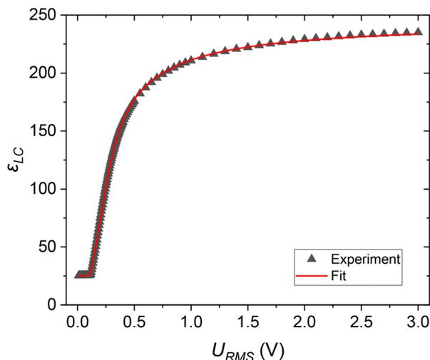
Fig. 7 Voltage dependence of the dielectric permittivity of the LC layer measured in the N phase at  $T = 78.5$  °C and  $f = 1.5$  kHz. The solid line represents the fit using eqn (3) and (4) with fitting parameters:  $U_{th} = 0.105$  V,  $\gamma = 8.678$ ,  $\kappa = 2.03$  ( $K_{11} = 2.18$  pN,  $K_{33} = 6.62$  pN).
