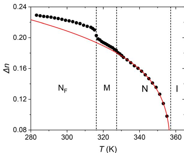
Fig. 2 Temperature dependence of birefringence ( $\Delta n$ ) in the liquid crystalline phases of the studied material determined at  $\lambda = 545 \text{ nm}$ . Black circles correspond to experimental data, while the solid line represents the theoretical fitting according to eqn (5).
