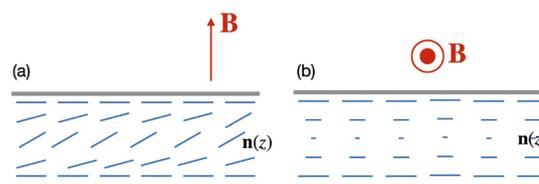
Fig. 6 Schematic representation of the measurement geometries for the splay (a) and twist (b) elastic constants using the magnetic Fréedericksz transition.  $\mathbf{n}$  and  $\mathbf{B}$  are the nematic director and the magnetic field, respectively. Strong planar anchoring condition is assumed.
