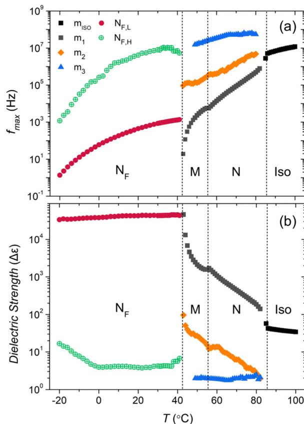
Fig. 5 (a) Temperature dependence of the relaxation frequency maxima ( $f_{\max}$ ) and (b) the dielectric strengths ( $\Delta\epsilon$ ) of the recorded relaxation mechanisms, obtained through fitting of the dielectric spectra with eqn (1).
