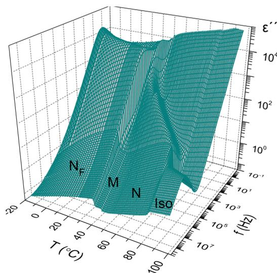
Fig. 4 3D plot of the imaginary part of the complex dielectric permittivity ( $\epsilon''$ ) as a function of temperature and frequency measured in 50  $\mu\text{m}$  thick parallel plate capacitor with untreated gold-plated brass electrodes.
