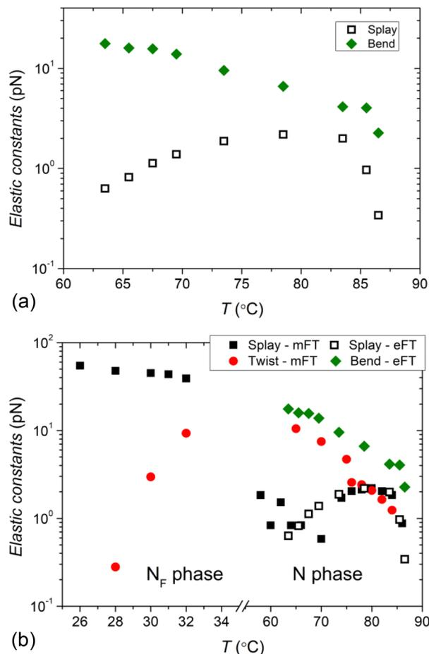
Fig. 9 Elastic constants in the N and N<sub>F</sub> phases: (a) the splay ( $K_{11}$ ) and bend ( $K_{33}$ ) elastic constants in the N phase determined by eFT and fitting the dielectric permittivity  $\epsilon_{LC}(U)$  with eqn (3) and (4). (b) Comparison of the elastic constants determined using the mFT and eFT.
