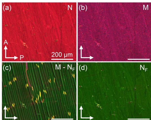
Fig. 1 Polarising optical microscopy textures of the studied compound in a 6  $\mu\text{m}$  thick planar cell with parallel rubbing: (a) N phase at 60  $^{\circ}\text{C}$ , (b) M phase at 46.4  $^{\circ}\text{C}$ , (c)  $\text{N}_\text{F}$  phase at 38.8  $^{\circ}\text{C}$  and (d)  $\text{N}_\text{F}$  phase at 28  $^{\circ}\text{C}$ . The rubbing direction forms an angle of 15 $^{\circ}$  with the analyser. The white bar is 200  $\mu\text{m}$ .
