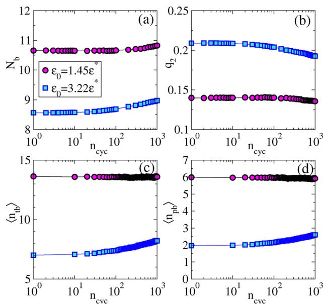
**Fig. 4** Microscopic structural analysis of sheared gel (simulation),  $\gamma_{\text{max}} = 0.04$ . (a) Coordination number  $N_b$  for increasing shear  $n_{\text{cyc}}$ . (b) Bond orientation order parameter  $q_2$ . (c and d) TCC analysis showing the number of trigonal bipyramids and pentagonal bipyramids in which the particles participate. (These results may be compared with Fig. 2.)
