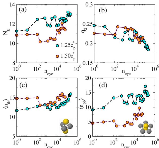
Fig. 2 Microscopic structural analysis of sheared gel (experiment). (a) Coordination number  $N_b$  as a function of the number of shear cycles  $n_{\text{cyc}}$ . (b) Two-fold bond orientation order parameter. (c and d) TCC analysis, showing the number of trigonal bipyramids and pentagonal bipyramids in which the particles participate. Insets show the relevant clusters. See Fig. 4 for a similar analysis of simulation data.
