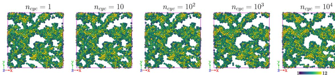
Fig. 7 Snapshot of the gel structure as shearing takes place. The parameters are those of Fig. 6 [ $\epsilon = 3.22\epsilon^*$ ,  $\gamma_{\max} = 0.035$ ] so the system is strain-hardening from  $n_{\text{cyc}} = 10^2$ – $10^3$  and softening from  $10^3$ – $10^4$ , although the structural changes are subtle. The region shown has size  $L \times L \times Z$  with  $Z = 8/$  (similar to Fig. 5), the colouring shows the co-ordination number (similar to Fig. 1).
