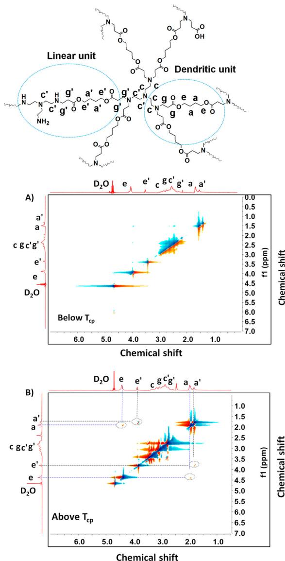
Fig. 5 (A) NOESY spectrum of PAE-TREN in D<sub>2</sub>O at 20 °C (below its  $T_{cp}$  of ~36 °C) at a concentration of 1 wt%. (B) NOESY spectrum of PAE-TREN in D<sub>2</sub>O at 60 °C (above its  $T_{cp}$  of ~36 °C) at a concentration of 1 wt%.
