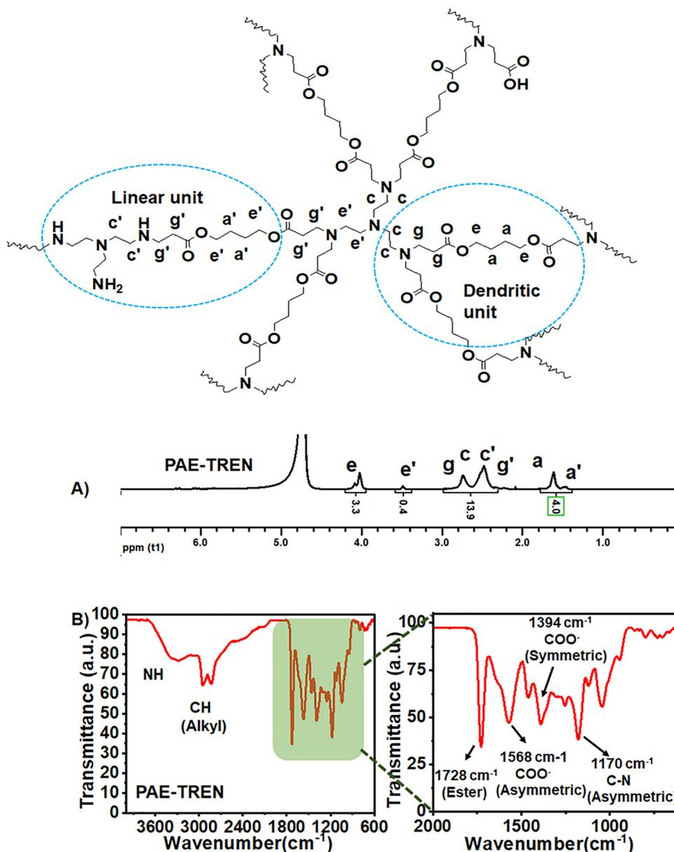
Fig. 1 (A) <sup>1</sup>H-NMR spectrum of PAE-TREN in D<sub>2</sub>O. (B) FTIR spectrum of PAE-TREN.
