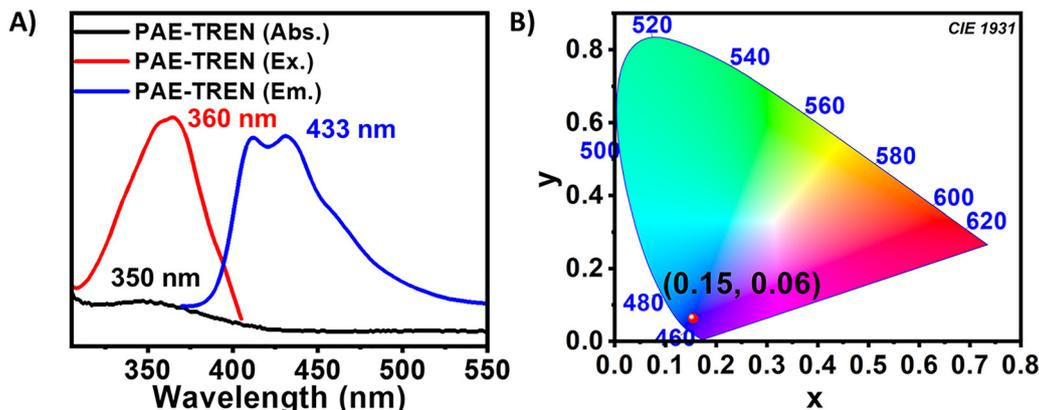
Fig. 6 (A) Excitation and emission spectra of PAE-TREN (0.1 wt%) with slit 2. (B) CIE 1931 chromaticity diagram of PAE-TREN (0.1 wt%) with slit 2.
