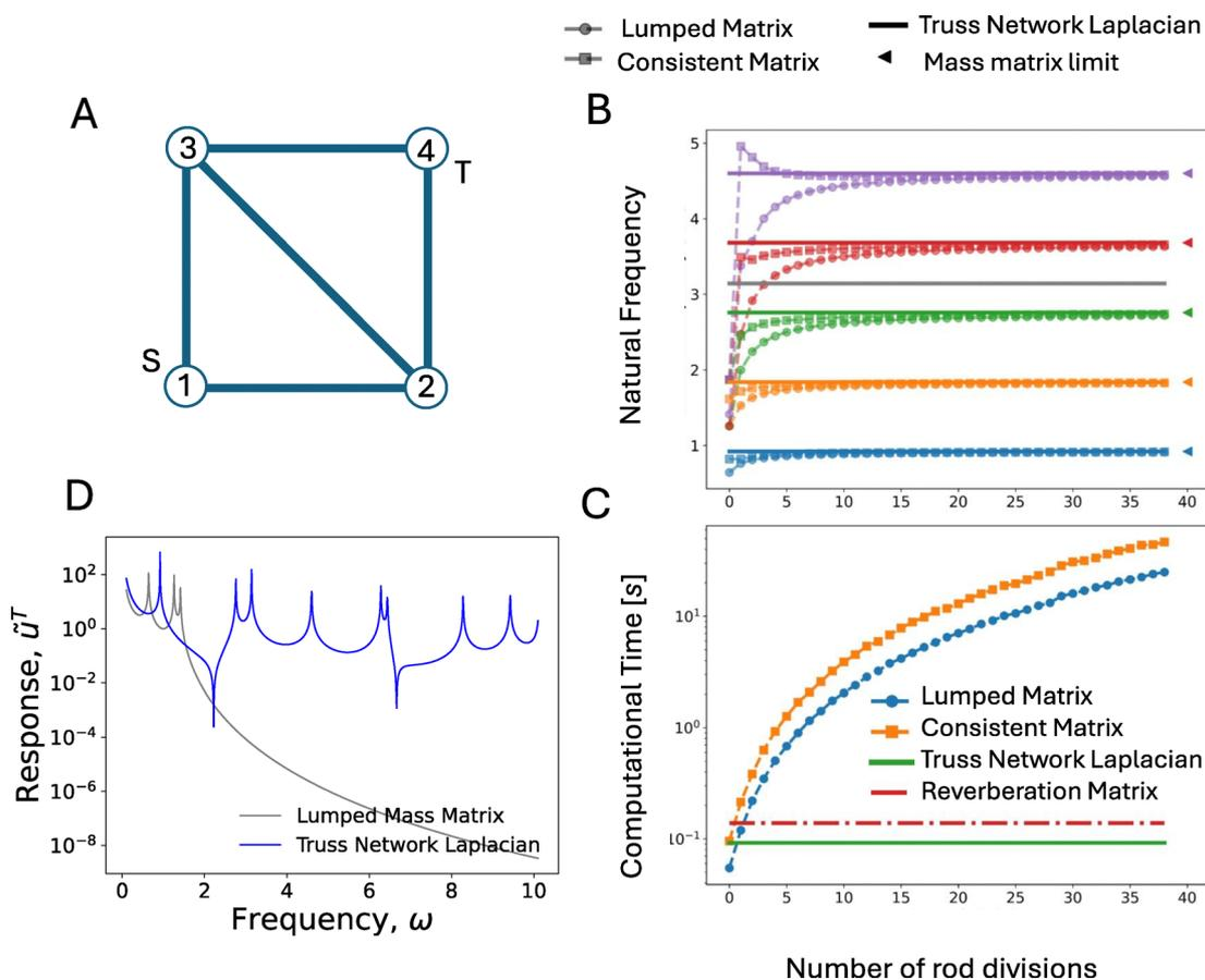
**Fig. 3** (A) Schematic of a square truss structure with a crossbar. (B) Comparison of natural frequencies computed using the truss network method and standard finite element methods for the square structure with a crossbar. The natural frequencies are plotted as a function of the number of subdivisions of the rods in the finite element methods. No subdivisions are necessary with the network Laplacian method to achieve the theoretical limit. (C)
