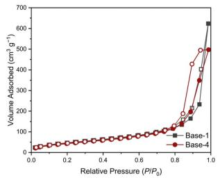
Fig. 8 Nitrogen adsorption isotherms of Base-1 and Base-4 samples collected at 77 K between  $0.025 \le P/P_0 \le 1.0$ . Adsorption branches are denoted by the filled symbols and desorption branches by the empty symbols
