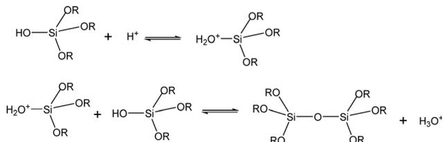
**Scheme 2** Schematic showing the acid-catalysed condensation reaction of TEOS, based on the reported procedure by Brinker *et al.*<sup>20</sup>
