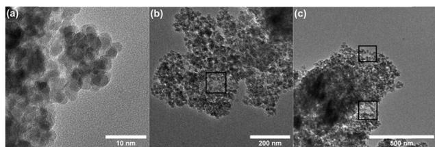
Fig. 5 TEM micrographs of Base-4 gel. Scale bar in (a) is 10 nm, in (b) is 200 nm, and in (c) is 500 nm.
