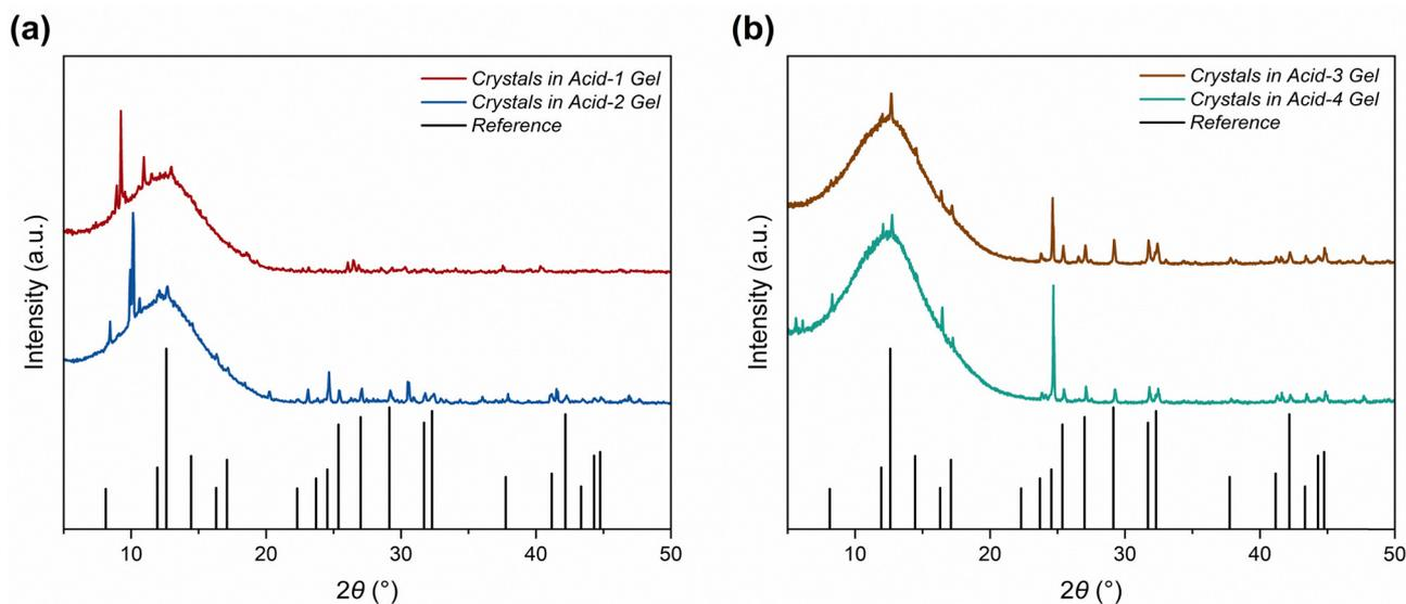
Fig. 10 PXRD patterns of (a) crystals grown in Acid-1 and Acid-2 gels; (b) crystals grown in Acid-3 and Acid-4 gels against ICSD reference #242181 pattern. Broad peak at  $2\theta \approx 12^\circ$  originates from the “low background” powder sample holder.
