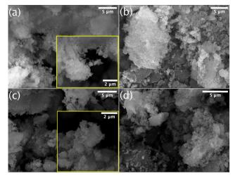
SEM micrographs of (a) Acid-2 gel, (b) Acid-3 gel, (c) and (d) Acid-4 gel. Scale bars in all four images are 5 μm, insets with 2 μm scale bars have been added to selected images for greater detail.
