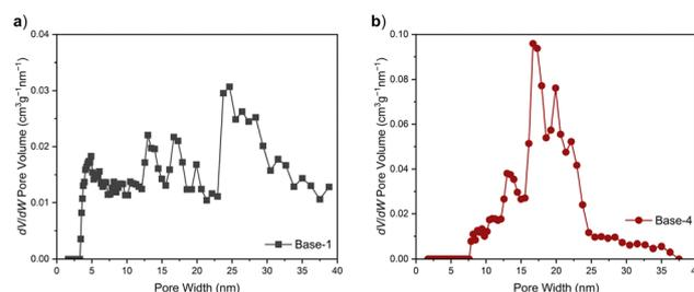
Fig. 9 Pore size distribution plots of (a) Base-1 and (b) Base-4 samples derived from the  $N_2$  isotherms using an NLDFT kernel, assuming a cylindrical pore model on a silica surface with  $N_2$  as the adsorbate at 77 K.
