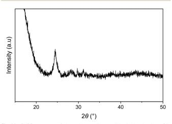
Fig. 11 PXRD pattern of the white-yellow solid obtained when Bil3 reagent is added to the Base-1 gel, collected between  $15-50^{\circ}$  ( $2\theta$ ). The broad peak at approximately 24° indicates the amorphous nature of the material
