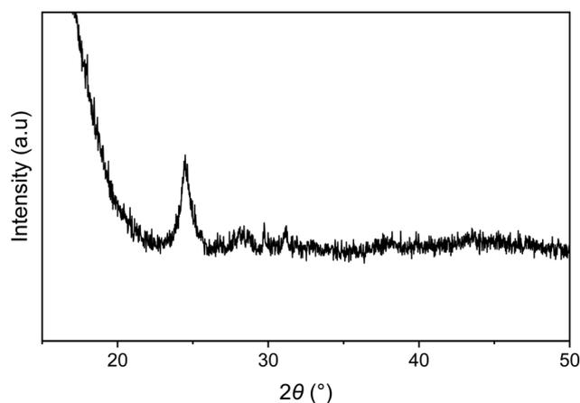
Fig. 11 PXRD pattern of the white-yellow solid obtained when  $\text{BiI}_3$  reagent is added to the Base-1 gel, collected between  $15\text{--}50^\circ$  ( $2\theta$ ). The broad peak at approximately  $24^\circ$  indicates the amorphous nature of the material.
