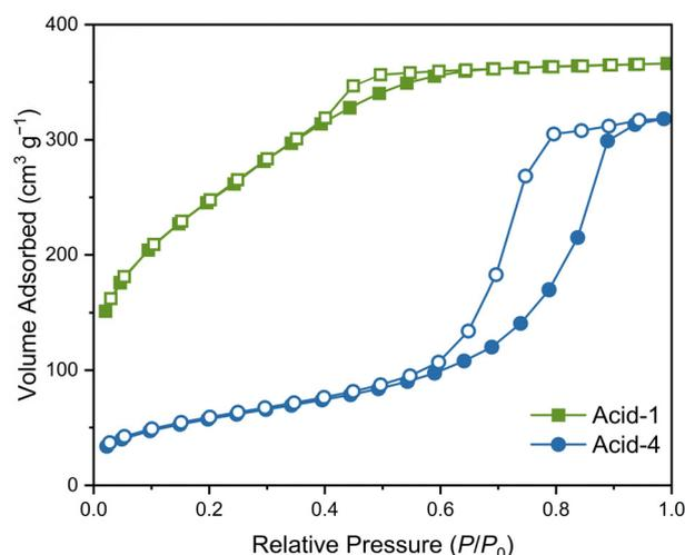
Fig. 6 Nitrogen adsorption and desorption isotherms of Acid-1 and Acid-4 samples collected at 77 K between  $0.025 \leq P/P_0 \leq 1.0$ . Adsorption branches are denoted by the filled symbols and desorption branches by the empty symbols.
