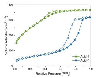
**Fig. 6** Nitrogen adsorption and desorption isotherms of Acid-1 and Acid-4 samples collected at 77 K between  $0.025 \le P/P_0 \le 1.0$ . Adsorption branches are denoted by the filled symbols and desorption branches by the empty symbols.
