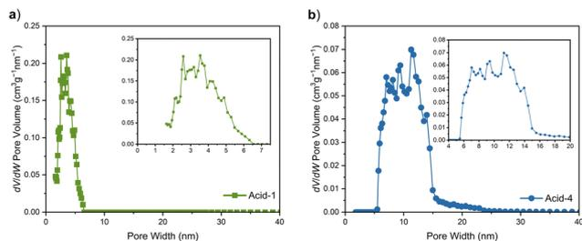
Fig. 7 Pore size distribution plots for (a) Acid-1 and (b) Acid-4 derived from the  $N_2$  isotherms using an NLDFT kernel, assuming a cylindrical pore model on a silica surface with  $N_2$  as the adsorbate at 77 K. The insets highlight the predominant pore sizes.
