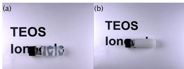
**Fig. 1** Digital photographs to show (a) acid-catalysed ionogel Acid-1 and (b) base-catalysed ionogel Base-1. Texts used to highlight transparency.
