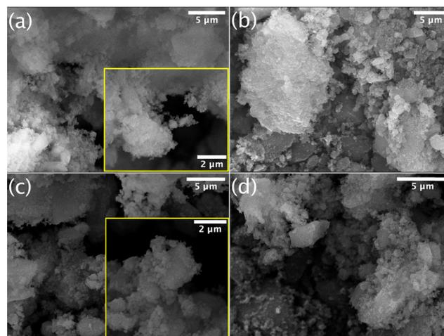
**Fig. 2** SEM micrographs of (a) Acid-2 gel, (b) Acid-3 gel, (c) and (d) Acid-4 gel. Scale bars in all four images are 5 μm, insets with 2 μm scale bars have been added to selected images for greater detail.
