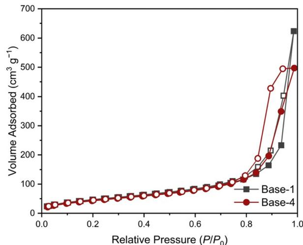
Fig. 8 Nitrogen adsorption isotherms of Base-1 and Base-4 samples collected at 77 K between  $0.025 \leq P/P_0 \leq 1.0$ . Adsorption branches are denoted by the filled symbols and desorption branches by the empty symbols.
