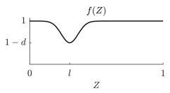
Fig. 2 Material damage is modelled with an inverted Gaussian f of magnitude d at Z = l.
