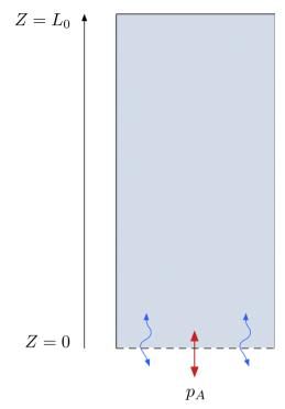
Fig. 1 We consider a poroelastic material of length  $L_0$  which is pulled at Z = 0 (red arrow) where it is also subject to ambient fluid pressure  $p_A$ , and fixed at  $Z = L_0$  with no deformation or flow. The blue arrows represent fluid flow. The material is shown in the reference configuration.
