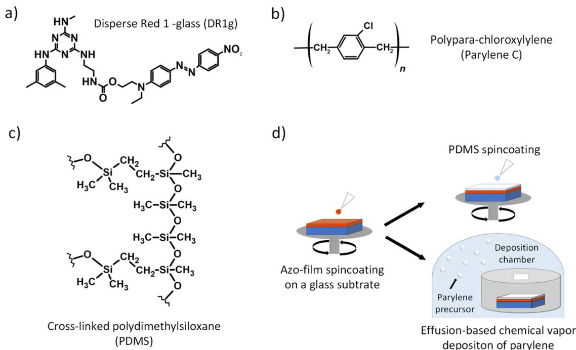
**Fig. 1** Chemical structures of (a) light-responsive DR1g, (b) parylene C and (c) cross-linked PDMS. (d) Schematic illustration of the sample fabrication process. First, azobenzene-based thin films are spin coated on a glass substrate. Subsequently, the PDMS coating is fabricated by spin coating and the parylene C coating is fabricated by effusion-based CVD.
