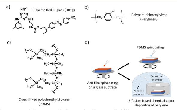
Fig. 1 Chemical structures of (a) light-responsive DR1g, (b) parylene C and (c) cross-linked PDMS. (d) Schematic illustration of the sample fabrication process. First, azobenzene-based thin films are spin coated on a glass substrate. Subsequently, the PDMS coating is fabricated by spin coating and the parylene C coating is fabricated by effusion-based CVD
