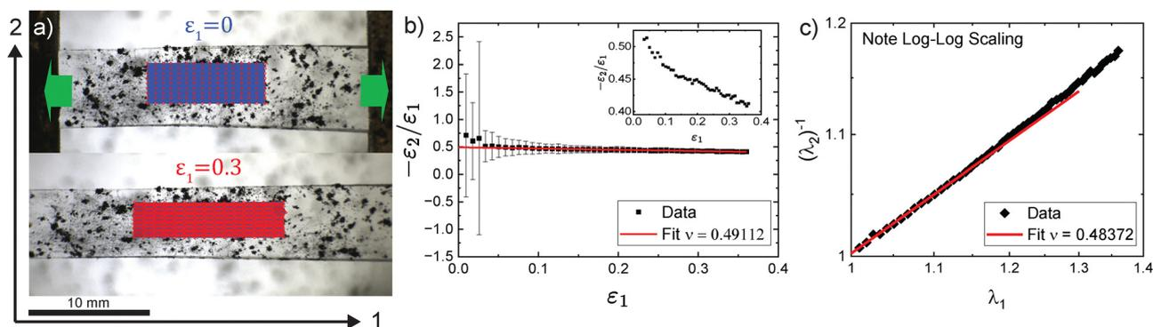
Fig. 2 (a) Images showing the stretching of rectangular strip with DIC overlay. (b) Plot of  $-\frac{\epsilon_2}{\epsilon_1}$  vs.  $\epsilon_1$  used in the DIC ratio method. (c) Log-log plot of  $(\lambda_2)^{-1}$  vs.  $\lambda_1$  used in the DIC scaling method.
