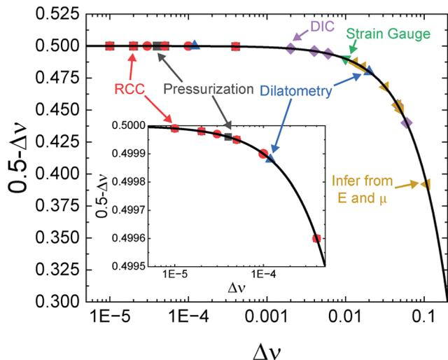
Fig. 1 Plot showing  $0.5 - \Delta\nu$  vs.  $\Delta\nu$  from literature data for RCC,<sup>7,8,24,25</sup> pressurization,<sup>23–25</sup> DIC,<sup>9,11,12</sup> strain gauge analysis,<sup>30</sup> dilatometry,<sup>17,30</sup> and inferred from  $E$  and  $\mu$ .<sup>28,29</sup>
