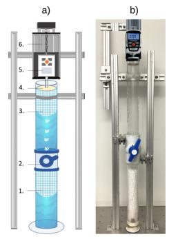
Fig. 5 (a) Sketch and (b) actual picture of the experimental system to measure the submerged Janssen effect for particles less dense than the liquid. The main components are: 1. particle reservoir, 2. valve, 3. polystyrene beads, 4. piston, 5. digital force sensor, 6. linear actuator.
