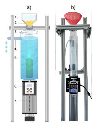
Fig. 1 (a) Sketch and (b) actual picture of the experimental setup used to measure the submerged Janssen effect for particles denser than the liquid. The components are: 1. funnel, 2. particles, 3. inner tube, 4. hose, 5. water container, 6. digital force sensor, 7. linear actuator.
