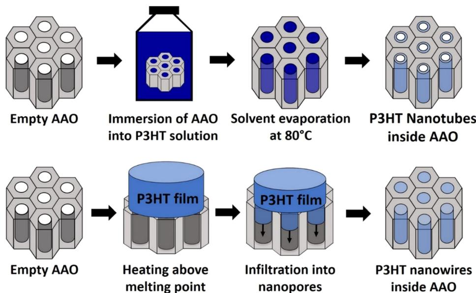
Fig. 1 Schematic representation of the preparation of polymer nanotubes (by solvent wetting, on the top) and polymer nanowires (by melt wetting, at the bottom), using AAO membranes as templates.
