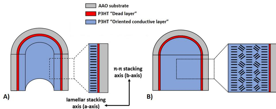
Fig. 7 Schematic representation of the cross-section of a nanopore containing P3HT nanotubes (A) and nanowires (B) showing the interplay between orientation effects and interfacial interactions. These effects lead to changes by order of magnitude in the conductivity value of P3HT nanotubes.
