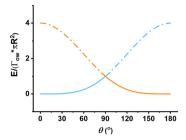
Fig. 2 The energy required to remove a particle from the interface. The blue curve represents moving the particle into the water phase, the orange curve represents moving the particle into the oil phase.
