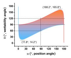
Fig. 6 Graph plotted from eqn (8). This graph is used to find the  $\alpha-\theta$ pairs that make the energy consumption of removing a particle from the interface equal to the thermal energy at T = 295 K (the blue and orange curves), or larger than the thermal energy (shaded area). Here it is assumed that  $\Gamma_{\text{ow}} = 50 \text{ mN m}^{-1} \text{ and } R = 100 \text{ nm}.$
