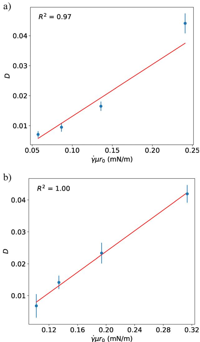
Fig. 4 Deformation,  $D$ , plotted as a function of  $\dot{\gamma}\mu r_0$  for flow tests in which (a)  $\chi = 1.39 \times 10^{-2}$  and (b)  $\chi = 1 \times 10^{-3}$ . In each plot the red line is a linear fit to the data, with slope  $1/\sigma$ . In (a),  $\sigma = 5.78 \pm 0.53 \text{ mN m}^{-1}$ , and in (b),  $\sigma = 6.28 \pm 0.03 \text{ mN m}^{-1}$ . The error bars on the data points in each plot indicate the standard deviation of the plateaus in Fig. 3a and b, respectively.
