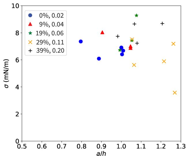
Fig. 7 Surface tension,  $\sigma$ , as a function of confinement, droplet diameter  $a$  divided by channel height,  $h$ . Measurements are obtained from steady deformation in stacked constrictions, with Span 80  $\chi = 10^{-2}$  and various amounts of PEGDA. The legend gives  $c$ , in volume %, and  $\lambda$ .
