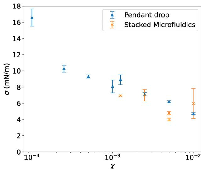
Fig. 8 Surface tension  $\sigma$  of oil drops in water as a function of SDS mole fraction  $\chi$  using the pendant drop method (blue) and stacked steady fluidics device (orange). The error bars on the pendant drop data represent the standard deviation of at least 7 measurements for each value of  $\chi$ ; error bars on the fluidics data represent standard errors in the linear fit, as described in Fig. 4.
