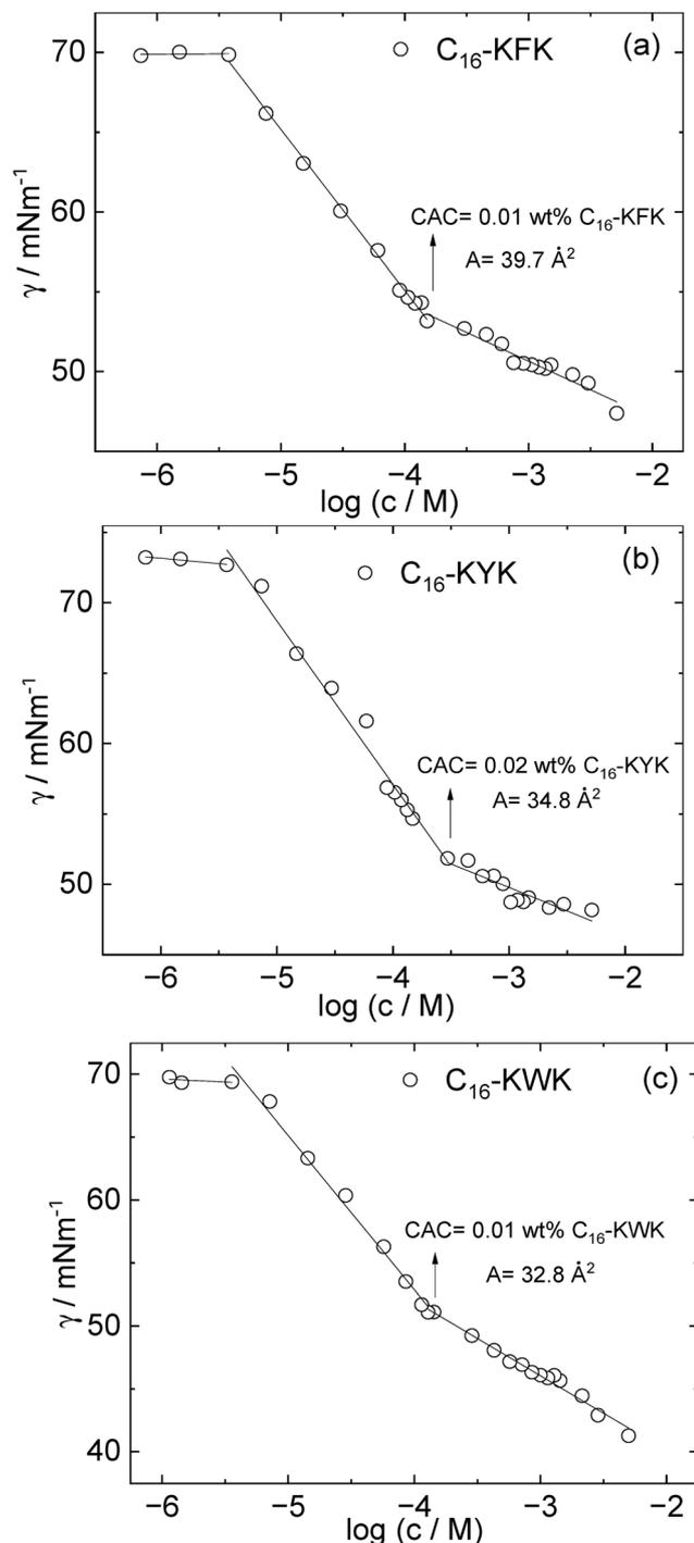
Fig. 7 Surface tension data (native pH). Langmuir adsorption isotherms for (a)  $C_{16}$ -KFK, (b)  $C_{16}$ -KYK and (c)  $C_{16}$ -KWK. Indicated are values of the CAC from the break points and the areas per molecule  $A$  from the slope of the lines below the CAC using the Langmuir adsorption isotherm equation (eqn (1) and (2)).
