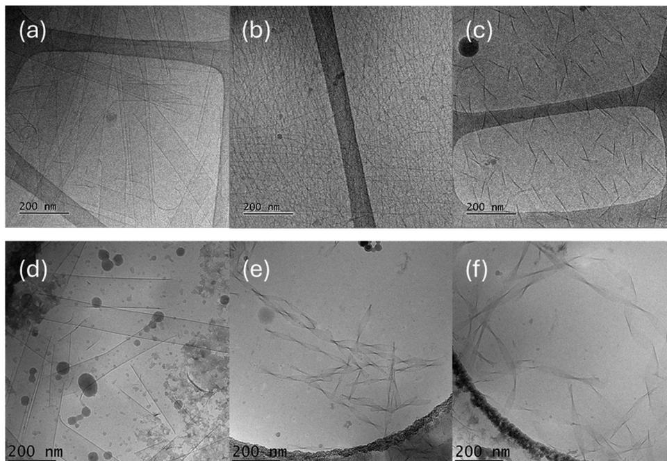
Fig. 1 Cryo-TEM images for 1 wt% samples at native pH (pH 2): (a) C<sub>16</sub>-KFK, (b) C<sub>16</sub>-KWK, (c) C<sub>16</sub>-KYK, and at pH 8: (d) C<sub>16</sub>-KFK, (e) C<sub>16</sub>-KWK, (f) C<sub>16</sub>-KYK.
