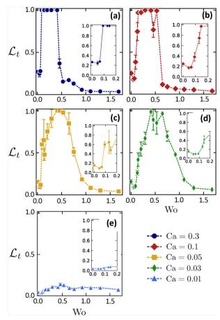
Fig. 12 Similar to Fig. 6, however for the wider channels (w/a = 7.33 and h/a = 1.5) and  $\phi = 12.00\%$ . Here,  $\mathcal{L}_t = 1$  corresponds to perfect triple-file trains as shown in Fig. 11a.
