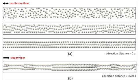
Fig. 11 (a) Progressive snapshots of hydrodynamic ordering in the wider channel (w/a = 7.33 and h/a = 1.5) with oscillatory flow leading to triple-file trains. The conditions are Wo = 0.194, Ca = 0.3, and  $\phi$  = 12.00% (number of particles = 210). The top image corresponds to the initial state. (b) The final particle configuration for an equivalent system in steady flow (Wo = 0).
