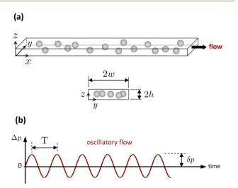
Fig. 1 (a) Schematic of simulation domain. The cross-sectional channel dimensions are  $2w \times 2h$ , and flow is in the x-direction. (b) Oscillatory flow is realized using a harmonic pressure gradient  $\Delta p$  (equivalent to the body force density  $F_x^b$ ) in the x-direction with an amplitude  $\delta p$  and time period T. For all oscillatory flow simulations herein, the  $\delta p$  value is chosen such that  $Re_{xyy} = \pm 1$
