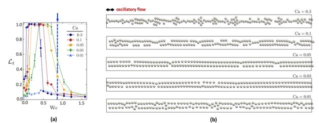
Fig. 9 Hydrodynamic ordering for Wo = 0.87 with varying Ca. (a) The full data set (also shown in Fig. 7a) with an arrow and dashed line indicating the conditions associated with the simulation snapshots shown in (b). At this value of Wo, the ordering is best for Ca = 0.03 and 0.05. The ordering diminishes for higher deformability (Ca = 0.1 and 0.3) and also lower deformability (Ca = 0.01).
