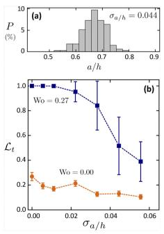
Fig. 15 (a) Histogram of the distribution of reduced particle radius (a/h) in a polydisperse suspension with a standard deviation of  $\sigma_{a/h}$  = 0.044. (b) Order parameter  $\mathcal{L}_l$  versus  $\sigma_{a/h}$  for oscillatory flow (Wo = 0.27) and steady flow (Wo = 0). For this data, Ca = 0.3,  $\phi$  = 10.66%, and the channel dimensions are w/a = 5.5 and h/a = 1.5. Note:  $\sigma_{a/h} = 0$  corresponds to a monodisperse suspension.
