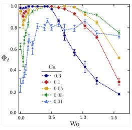
Fig. 10 Order parameter  $\Phi_{tr}$  representing the fraction of particles belonging to a train, versus Wo for each Ca value. For steady flow conditions (Wo = 0), increasing Ca results in increased  $\Phi_t$ . However, increasing Wo leads to deformability-dependent trends. For the softest particles (Ca = 0.3), there is a marked decrease in  $\Phi_t$  for Wo > 0.5. On the other hand, for the stiffest particles (Ca = 0.01), there is a marked increase in  $\Phi_t$  with increasing Wo.
