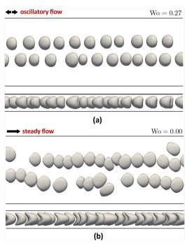
Fig. 17 Close-up views of the shaded boxes in Fig. 16, including topdown and side views. These images better depict the variation in particle size. (a) Close-up image of particle configurations for Wo = 0.27 and  $\sigma_{a/h}$  = 0.0333. (b) Close-up image of particle configurations for Wo = 0.00 and  $\sigma_{a/h} = 0.0333$ .
