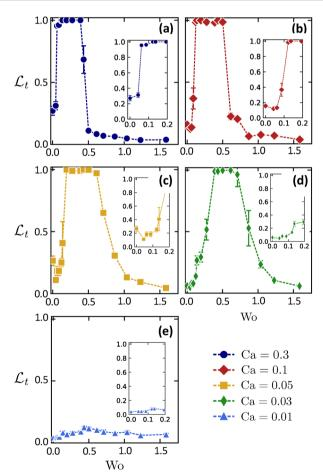
**Fig. 6** Order parameter  $\mathcal{L}_t$  versus Womersley number Wo for each of the Ca values. For each plot, the volume fraction is  $\phi=10.66\%$ , and the channel dimensions are w/a=5.5 and h/a=1.5. Insets show data values for Wo < 0.2 with the same axes labels. Steady flow corresponds to Wo = 0. The results suggest an optimal range of Wo for hydrodynamic ordering for each Ca value (with the exception of Ca = 0.01 shown in panel e).
