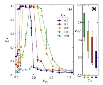
Fig. 7 (a) Each data set shown in Fig. 6 plotted together to show that the optimal range of Wo shifts to smaller values of Wo as particle deformability increases from Ca = 0.03 to Ca = 0.3. (b) Box plot showing the optimal range of Wo (designated as Wo\*) for Ca = [0.03, 0.05, 0.1, 0.3]. Note that Ca = 0.01 is not included in panel b due to a lack of ordering in this system.
