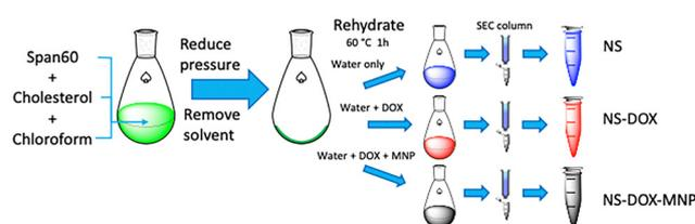
Fig. 3 A schematic representation of the niosome synthesis. NS, DOX, MNP and SEC stand for niosome, doxorubicin, magnetic nanoparticles and size exclusion respectively.
