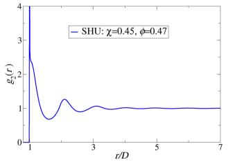
Fig. 7 The pair correlation function  $g_2(r)$  versus dimensionless distance r/D of 3D SHU sphere-packing ground states with a high value of  $\chi$ . Here, D is the hard-sphere diameter. We consider the ground states with  $\chi = 0.45$ , N = 4000,  $\phi = 0.47$ , and  $n_c = 500$ .
