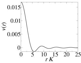
Fig. 1 The three-dimensional direct-space long-ranged pair potential v(r)versus the dimensionless distance rK associated with the Fourier transform  $\tilde{v}(k)$  that is unity for k < K and zero otherwise, i.e.,  $\tilde{v}(k) = v_0 \Theta(K - k)$ . We choose  $v_0 = 1$ . This pair potential will be used in our subsequent computations; see eqn (3) with d = 3
